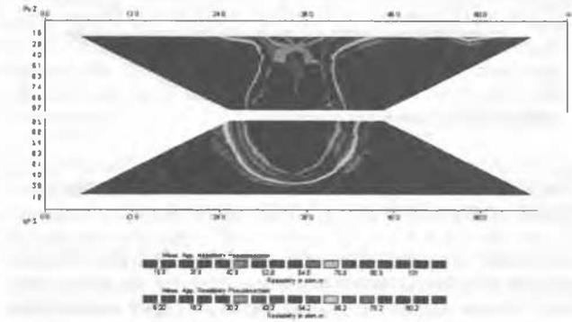
Fig. 5(a): Resistivity tomography image associated with 10 g/l (NaCl) contaminant infiltration into partially-saturated sand at 1g
