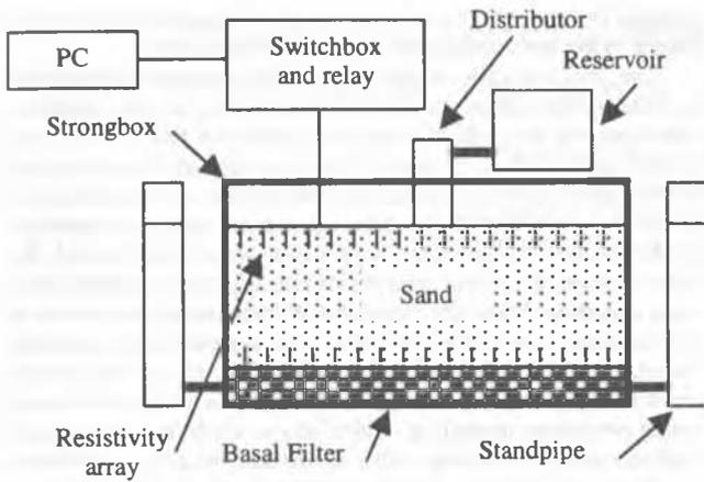
Figure 3: Centrifuge box and resistivity imaging equipment
