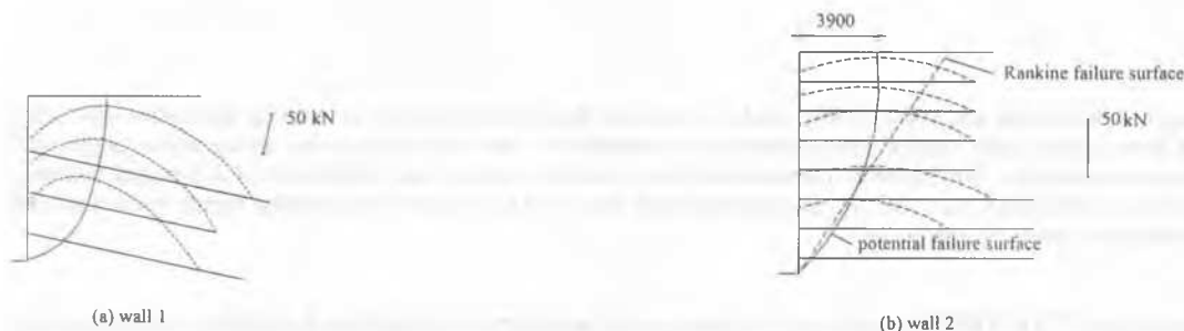
Figure 3 . Distribution of the axial forces and potential failure surface (wall 1 and wall 2 )
