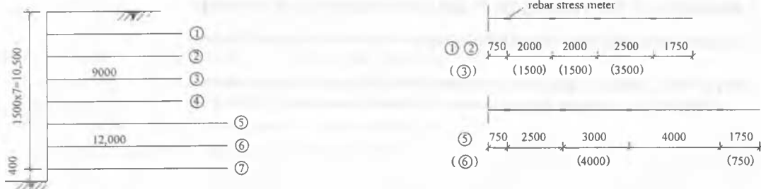
Figure 2. Cross-section of nailed wall 2 and rebar stress meters layout (mm)
