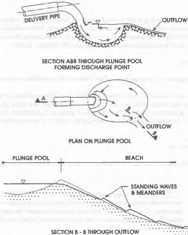
Figure 2. Geometry of plunge pool and initial part of tailings beach.
