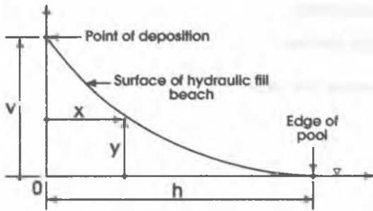
Figure 1. Basis for defining the shape of an hydraulic fill beach.
