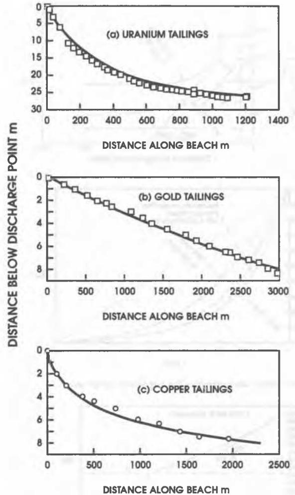
Figure 3. Comparison of observed and predicted tailing beach profiles for three types of tailings.
