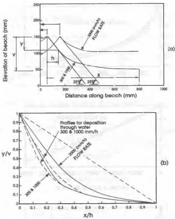
Figure 5. Beach characteristics for disposition under water.
