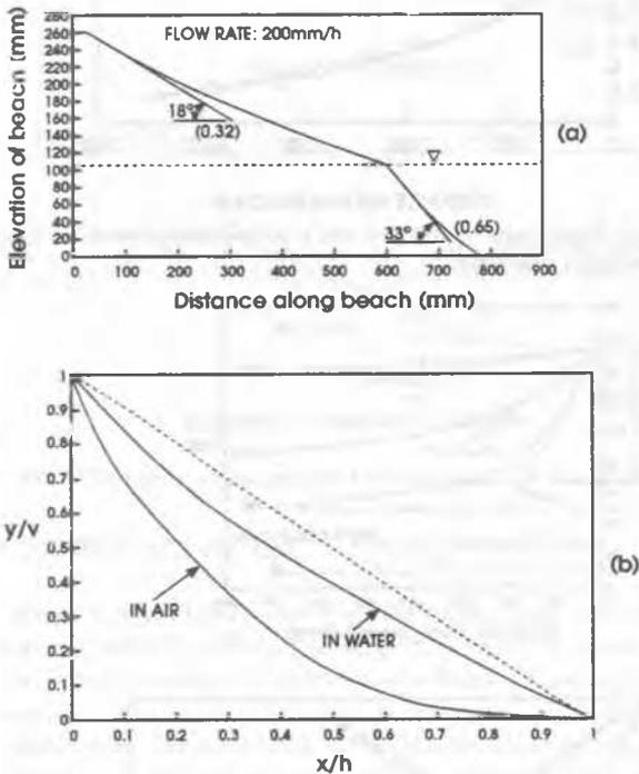
Figure 6. Beach characteristics for deposition in air, running into water - 100% sand.
