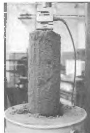
Figure 3. A complete sand-cement-waste column.
