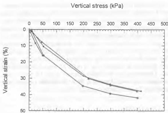
Figure 2 Results of four compression tests conducted on tire shreds (50x50mm<sup>2</sup>).
