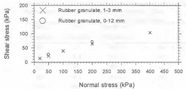
Figure 3 Failure values from shear tests conducted on rubber granulate, 1-3 mm and 0-12 mm respectively.
