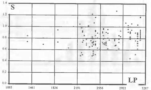
Figure 3. Settlement (S) ratio versus Loading Period (LP) in days
