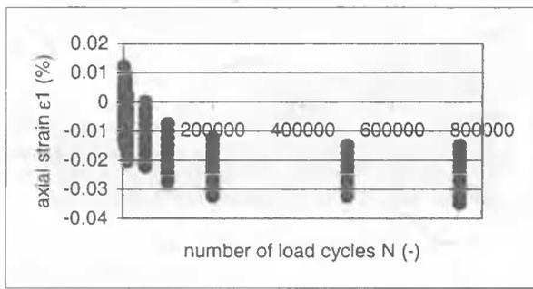
Figure 5. Cyclic response of the specimen with a curing time of 10 days
