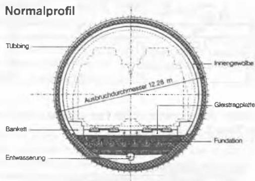
Figure 1 System of the tunnel.
