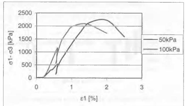
Figure 4. Stress-strain response of the stabilised marl
