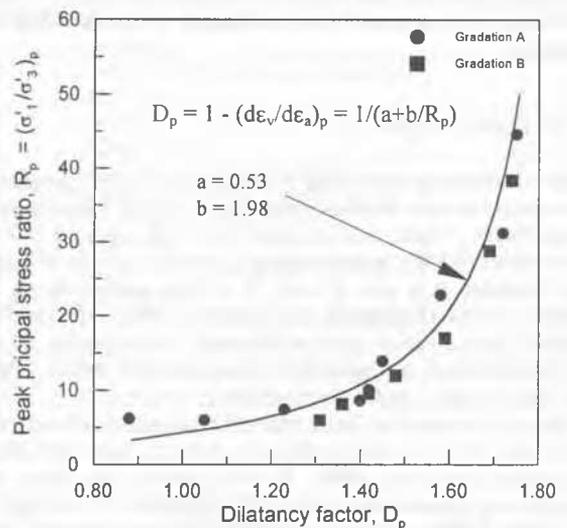
Fig. 5. The strength-dilatancy relationship for ballast aggregates
