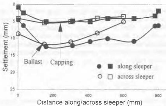
Fig. 9. Settlement of ballast and capping layer in dynamic testing (modified after Indraratna and Ionescu, 1999)
