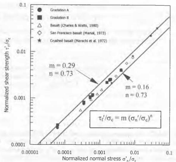
Fig. 4. Normalized stress-strength relationship for various aggregates (modified after Indraratna et al. 1993, 1998)
