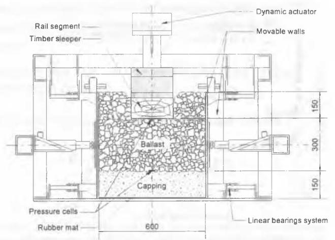
Fig. 7. Process simulation triaxial apparatus at University of Wollongong
