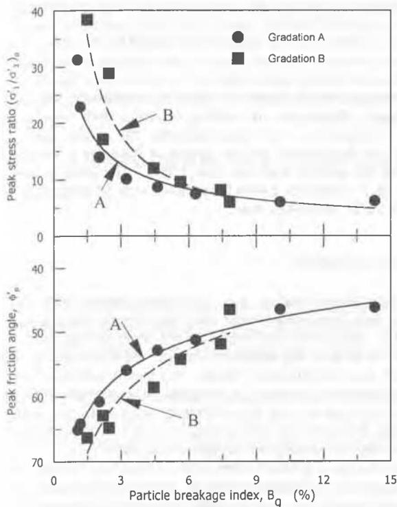
Fig. 6. Peak stress ratio, friction angle and particle breakage relation (modified after Indraratna et al. 1998)
