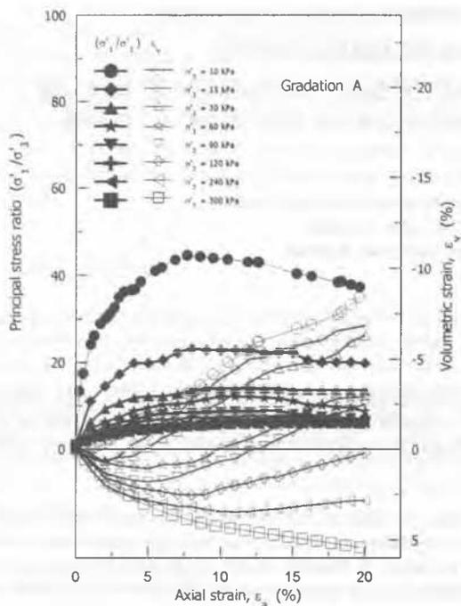
Fig. 2. Principal stress ratio and volumetric strain at various confining pressures (modified after Indraratna et al. 1998 with additional data)
