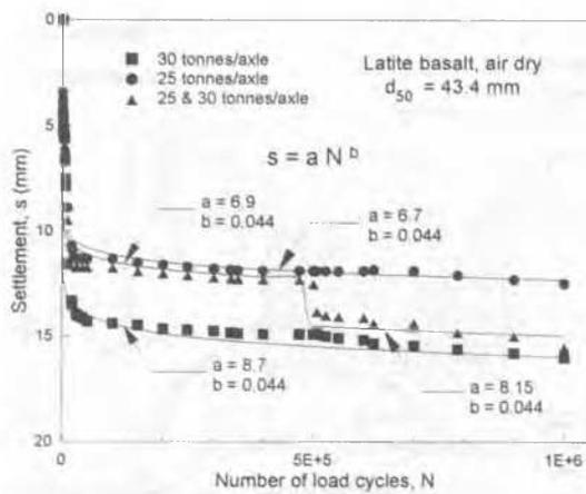
Fig. 8. Effect of load cycles and axle loads on settlement (after Indraratna and Ionescu, 1999)
