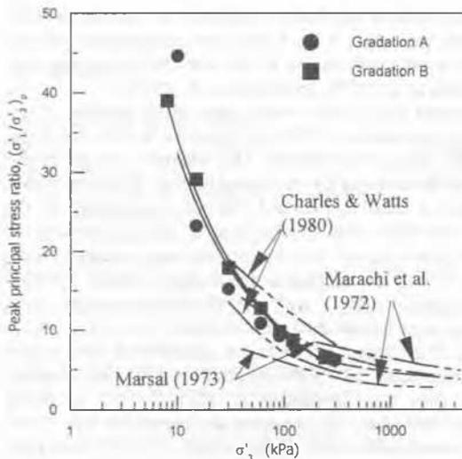
Fig. 3. Effect of confining pressure on peak stress ratio (modified after Indraratna et al. 1993, 1998)
