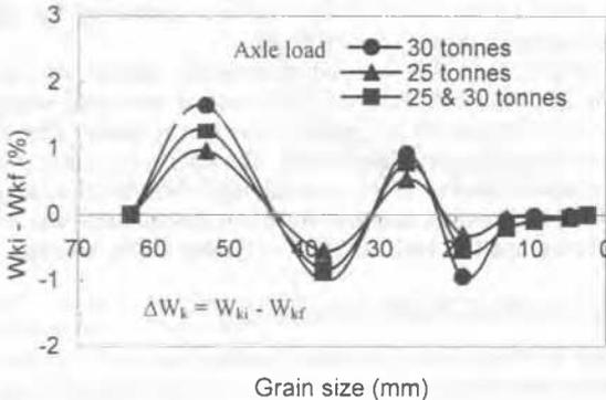
Fig. 10. Grain breakage in dynamic triaxial testing (modified after Indraratna and Ionescu, 1999)
