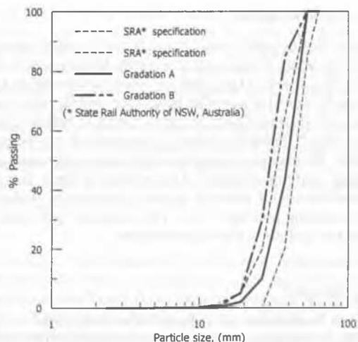
Fig. 1. Grain size distribution of railway ballast
