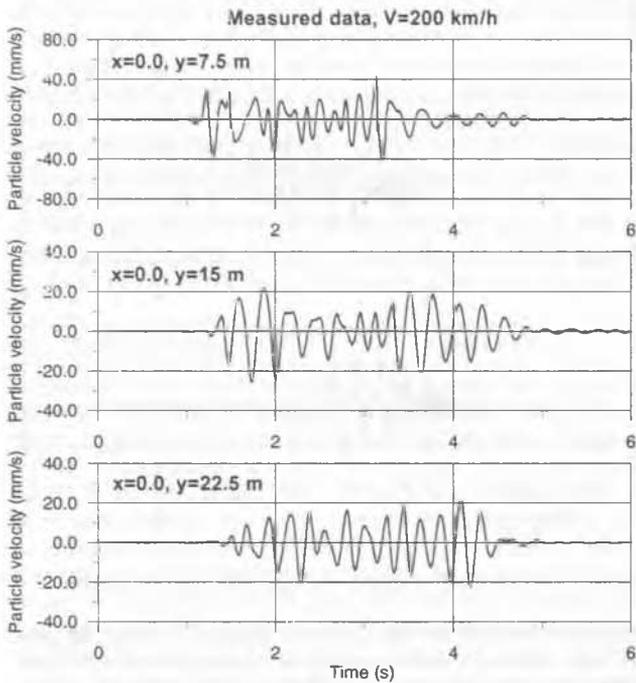
Figure 6. Measured track-side vibration for train speed 200 km/h
