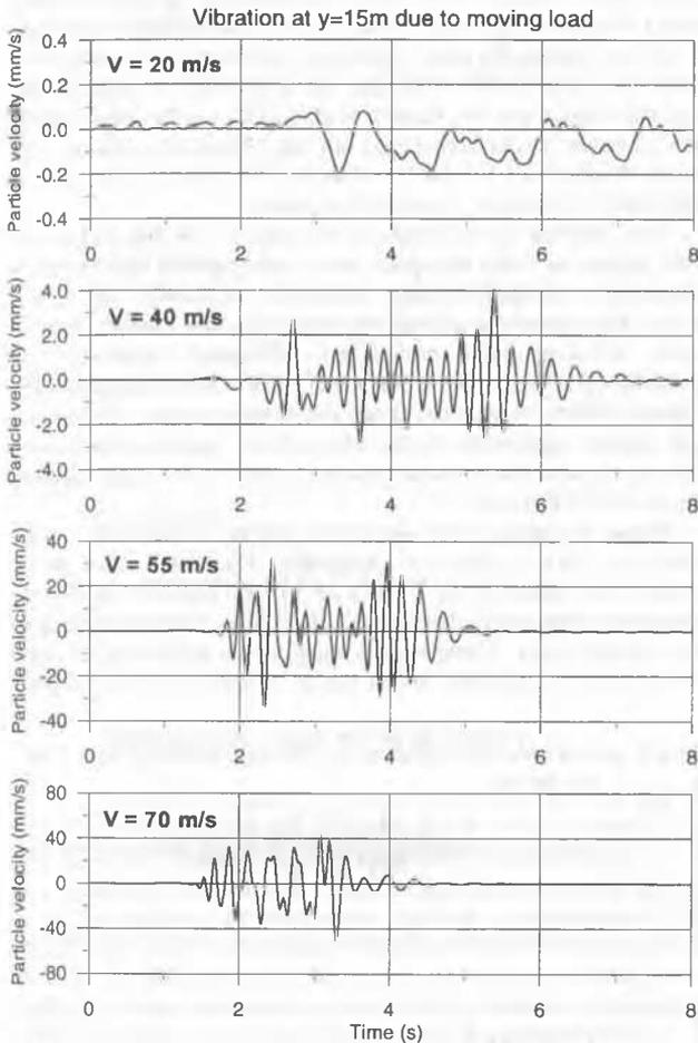
Figure 4. Simulated moving-load component of ground vibration
