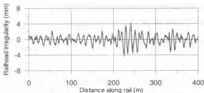
Figure 2. Typical rail irregularity profile at Ledsgaard test site
