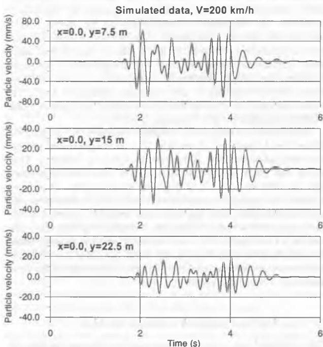
Figure 7. Simulated track-side vibration for train speed 200 km/h
