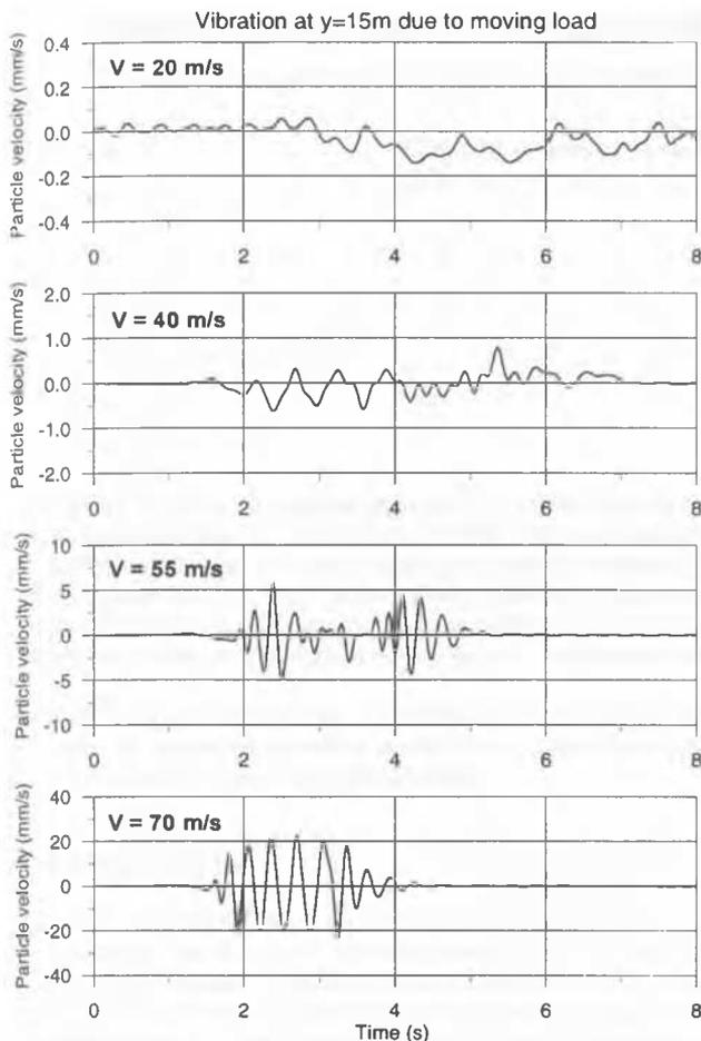
Figure 9. Simulated moving-load excitation of ground vibration for stiff track
