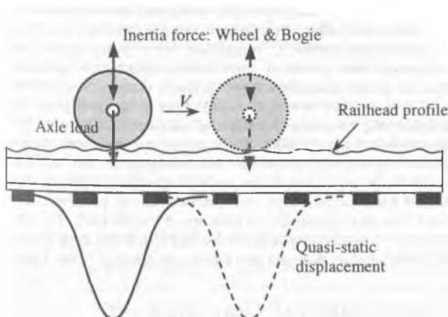
Figure 1. Schematic representation of railway excitation mechanisms
