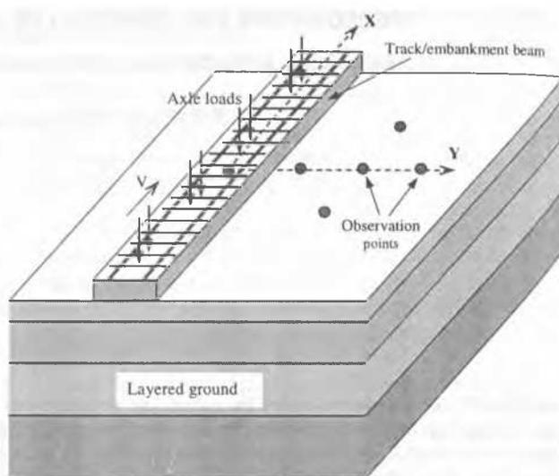
Figure 3. Elements of *VibTrain* calculation model
