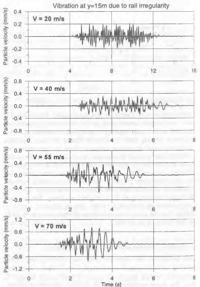
Figure 8. Simulated rail-irregularity component of ground vibration for stiff track
