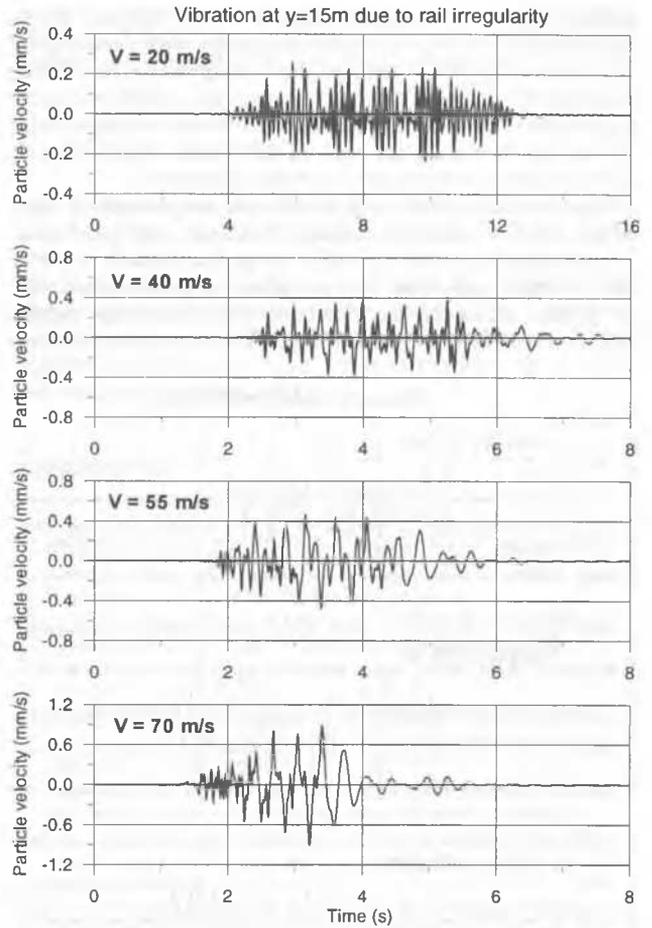
Figure 5. Simulated rail-irregularity component of ground vibration
