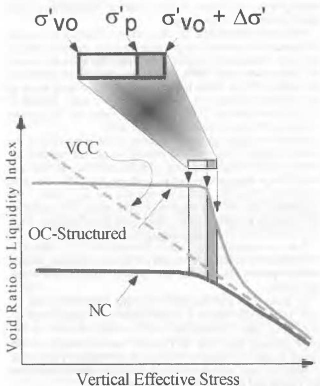
Figure 6. Conceptual view of the potential role of microfossils to explain alternating layer of consolidated and overconsolidated clays at Kansai airport (see also Locat and Tanaka 2000). VCC is the reference virgin compression curve (Bjerrum 1967, Locat and Lefebvre 1986).
