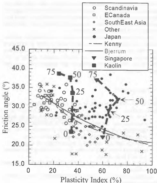
Figure 7. Effect of diatom on the measured friction angle of artificially prepared mixtures of kaolin and Singapore clay (modified after Shiwakoti *et al.* 2001).
