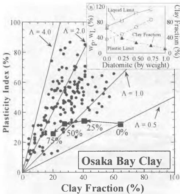
Figure 5. Impact of diatoms on the activity of a kaolin clay. The data from Osaka Bay are given in the background (modified from Tanaka and Locat 1999). In (b) are test results on mixtures of kaolin and diatomite used in the Activity Chart.
