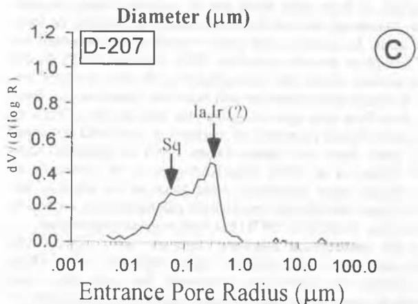
Figure 3. Distribution of diatoms in a consolidated sediment taken at a depth of 383 m at the site of Kansai airport (a), the grain size distribution (b) and the pore size distribution (c) with indications for skeletal porosity (Sq), intra- (Ia) and inter- (Ir)-aggregate pores.
