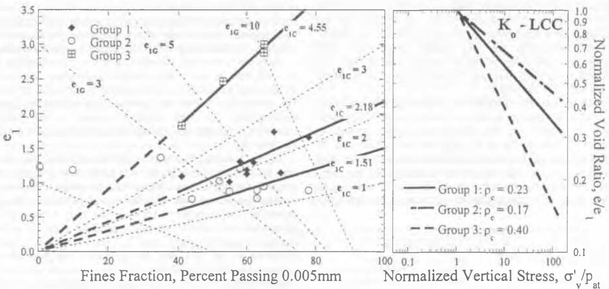
Figure 7: Compression parameters for silty clay materials as a function of clay fraction ( $<5\mu\text{m}$ ).
