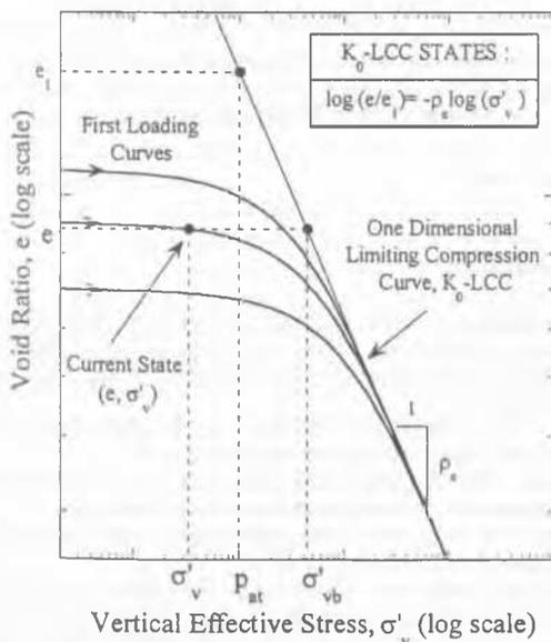
Figure 5. Idealized behavior of silty clays soils (modified from Pestana, 1994, Pestana & Whittle, 1995).
