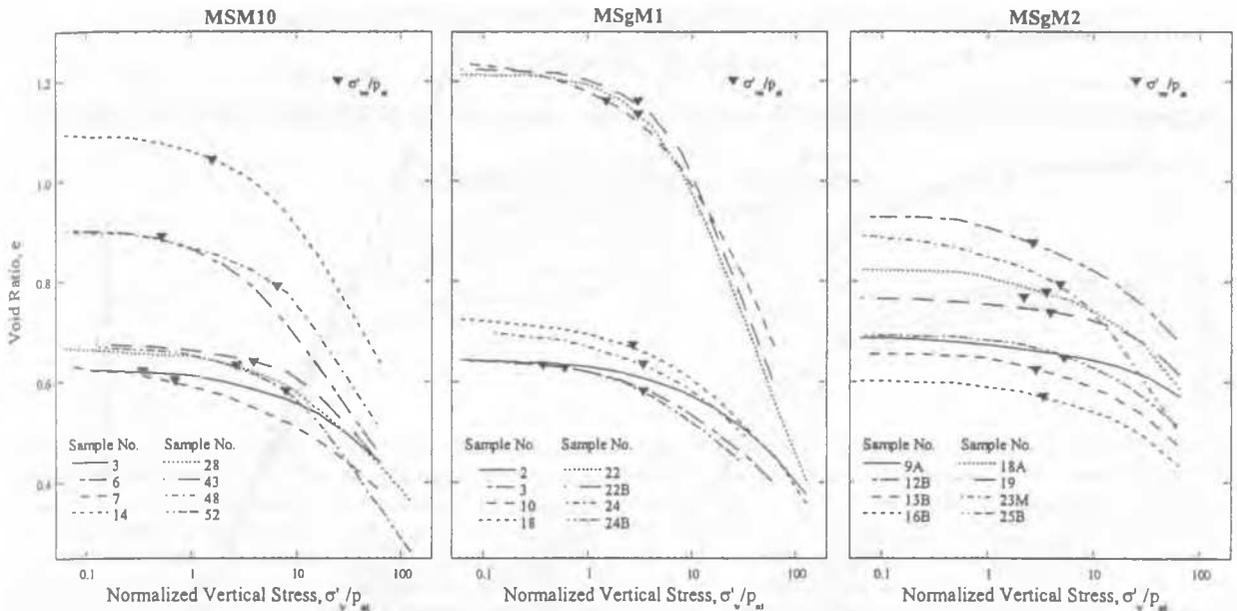
Figure 4. Oedometer compression curves for the soils at the Port of Malamocco test site.
