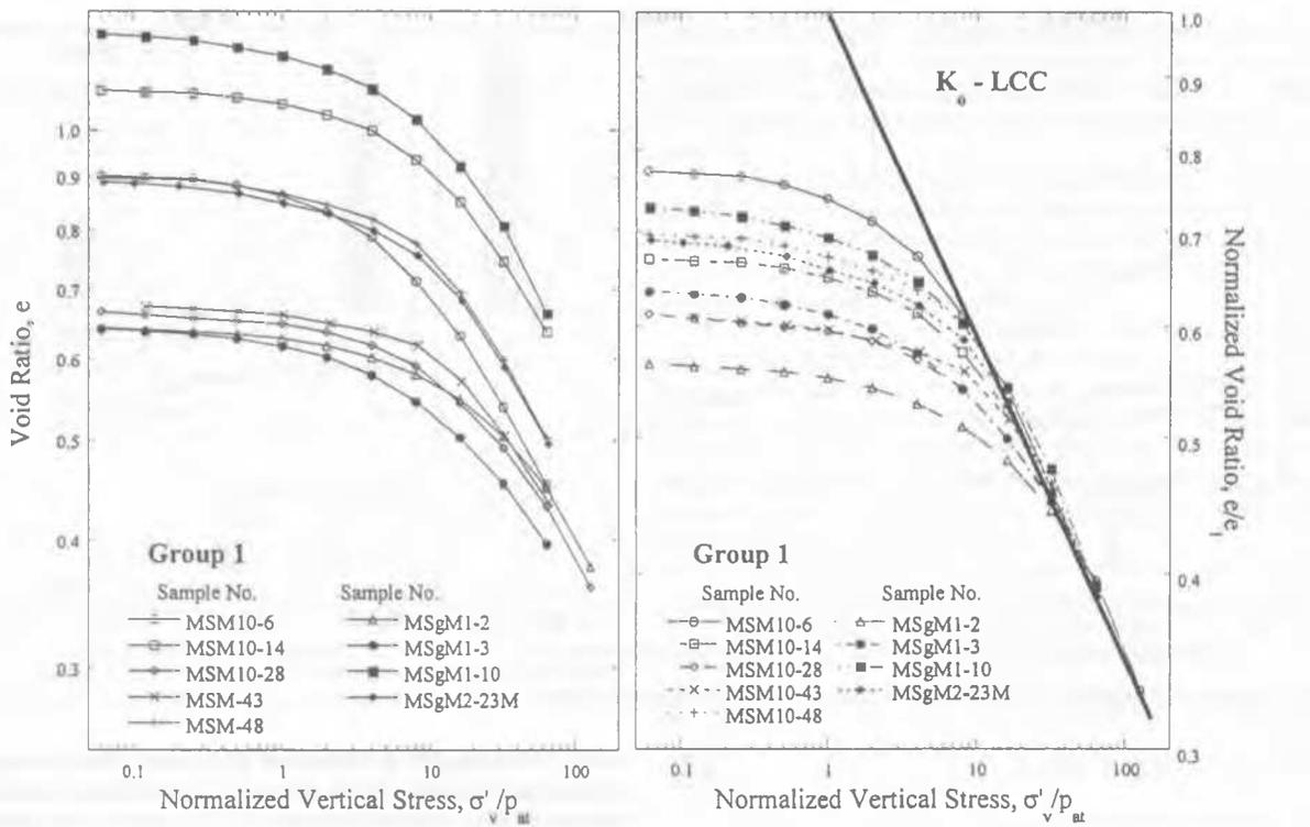
Figure 6: One dimensional compression curves and normalized response for silty clay materials.
