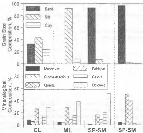
Figure 2. Comparison between grain size distribution and mineralogical composition of soils at Port of Malamocco test site.
