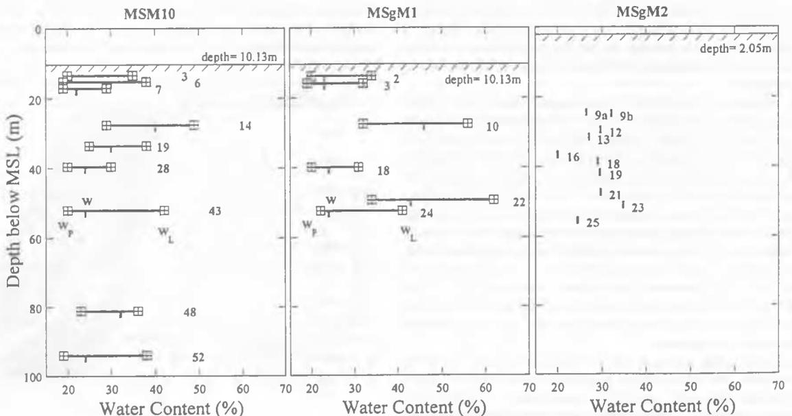
Figure 3. Profile of water content and index properties for soils at the Port of Malamocco test site.
