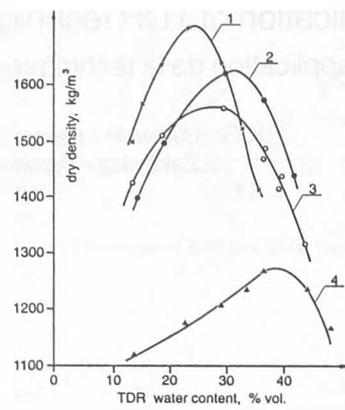
Figure 2. Compaction curves obtained with using TDR technique; 1, 2 and 3 - number of soils tested (silty clays), 4-ash.
