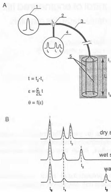
Figure 1. Principle of water content measurements by TDR technique; A-main components of reflectometer (1-oscilloscope screen, 2-T-connection, 3-feeder, 4-oscillogram, 5-bars), B - oscillograms.
