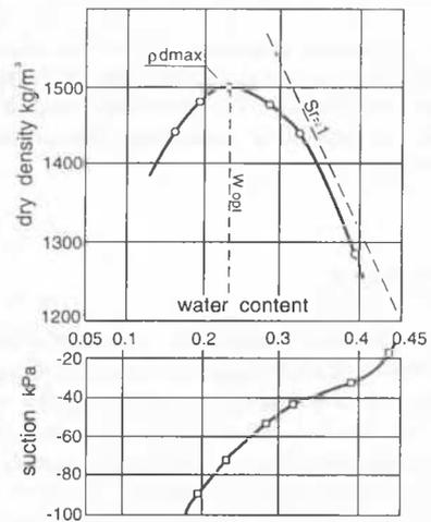
Figure 3. Nomograph for compaction control of clay.
