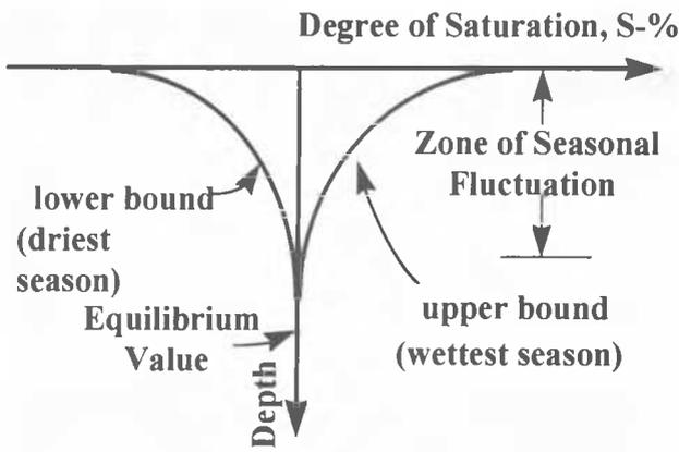
Figure 1. Schematic of Degree of Saturation Variation with Depth
