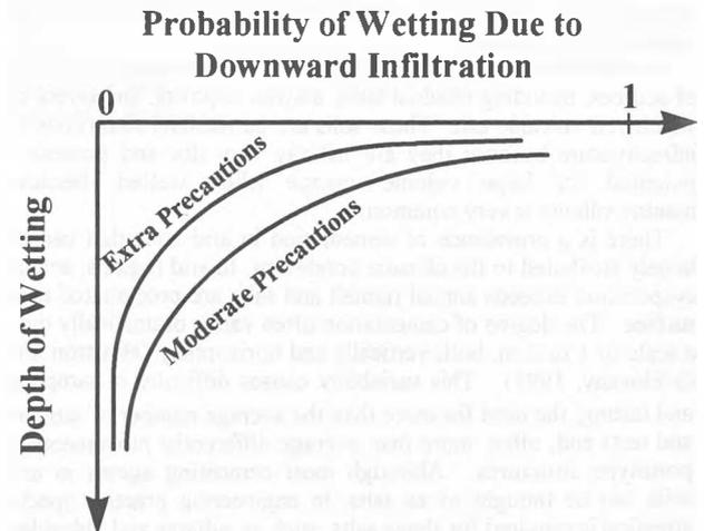
Figure 2. Schematic Variation of Probability of Wetting vs. Depth of Wetting
