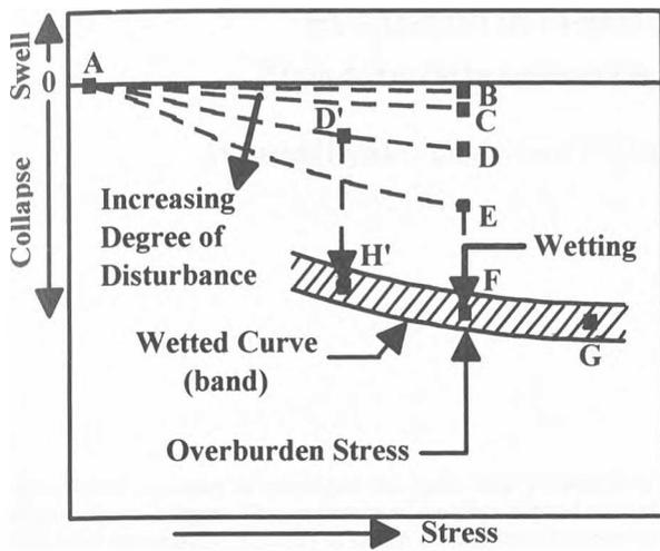
**Figure 3. Schematic of Response to Wetting for a Collapsible Soil**
