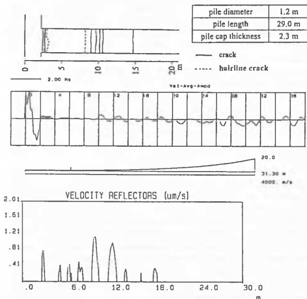
Figure 5: Comparison between PIT and BIP Data
