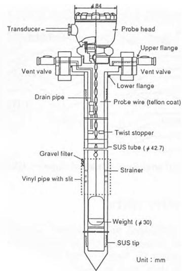
Figure 3: Schematic diagram of liquefaction sensor
