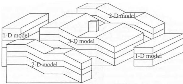
Figure 4: A typical analytical model of SuperFLUSH/3DC
