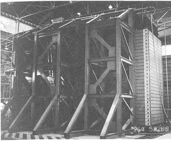
Figure 2: A view of the large-scale laminar shear box
