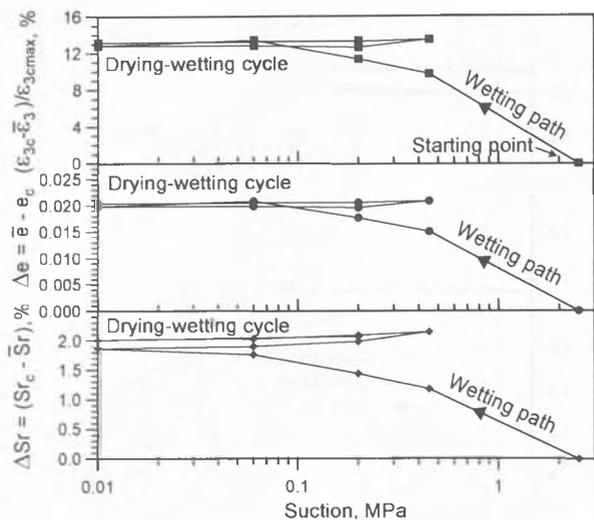
Figure 4. Differences between measured mid-height radial strains ( $\epsilon_{3c}$ ) and calculated mean value radial strains ( $\epsilon_3$ ) and their consequences in terms of void ratio and degree of saturation errors.
