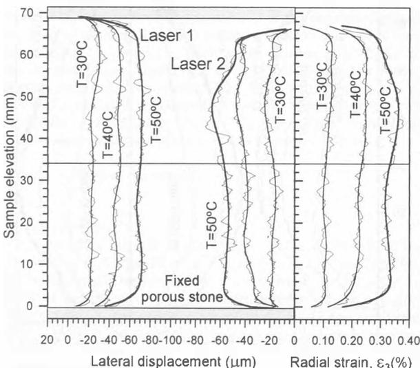
Figure 5. Progressive development of the lateral profiles of the specimen in a heating path ( $T_o=22^\circ\text{C}$  to  $T_f=50^\circ\text{C}$ ) under a constant suction of  $s=0.20$  MPa and an isotropic net mean stress of ( $\sigma_m - u_a$ )=1.00 MPa.
