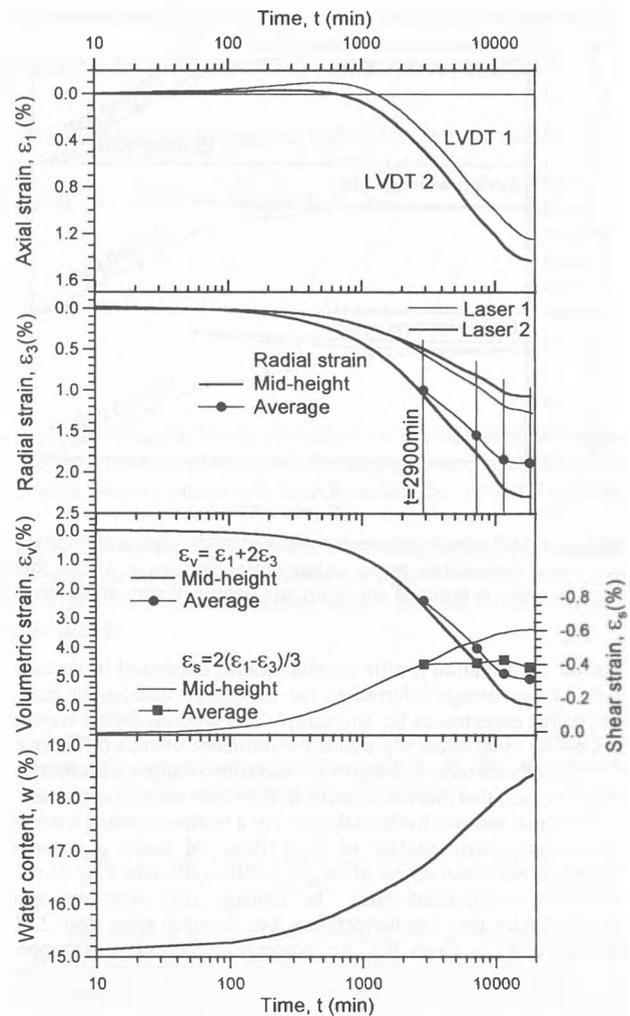
Figure 2. Time evolution of axial, radial, volumetric and shear strains and water volume change in a wetting path ( $\psi_o=2.5$  MPa to  $s=0.45$  MPa) under a constant isotropic net mean stress of  $(\sigma_m - u_a)=0.60$  MPa.
