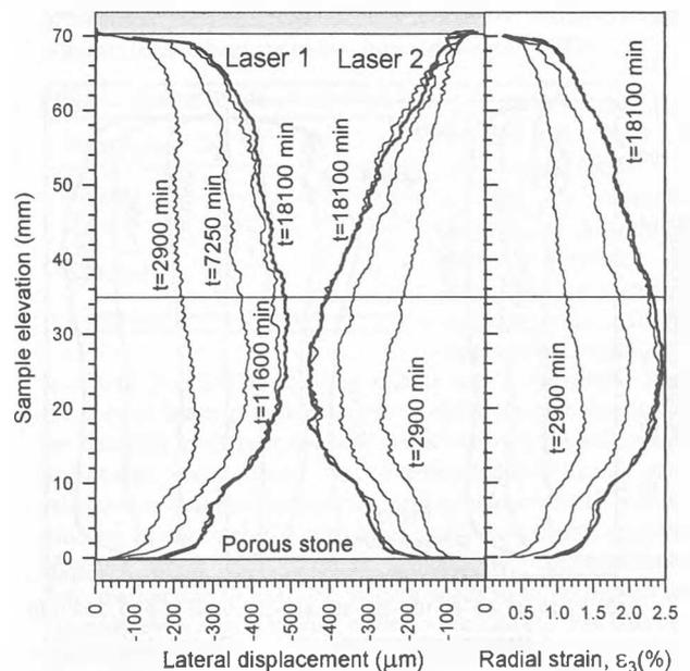
Figure 3. Progressive development of the lateral profiles of the specimen in a wetting path ( $\psi_o=2.5$  MPa to  $s=0.45$  MPa) under a constant isotropic net mean stress of  $(\sigma_m - u_a)=0.60$  MPa.
