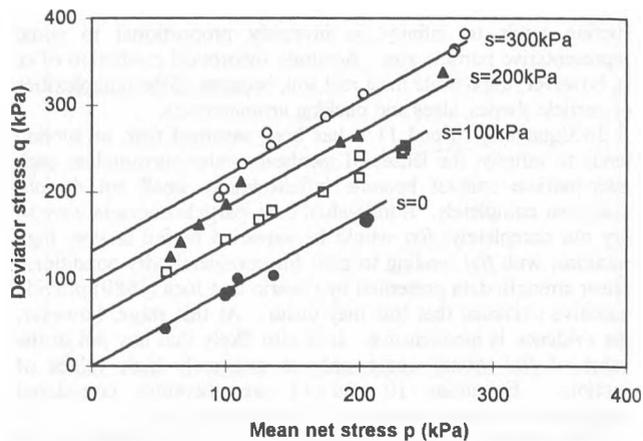
Fig. 3 Critical state data for compacted Speswhite kaolin
