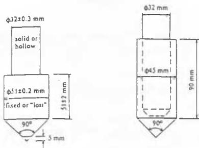
Fig 1 Dynamic probing equipment types DPB (left) and HfA.
