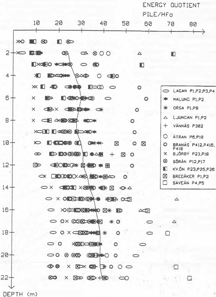
Fig. 5 Quotient between the necessary energies to drive the piles and the rods at 12 piling sites in Sweden.
