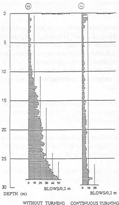
Fig.2 Comparison between sounding resistance at dynamic probing in sand with and without turning. (Bergdahl & Dahlberg, 1973)
