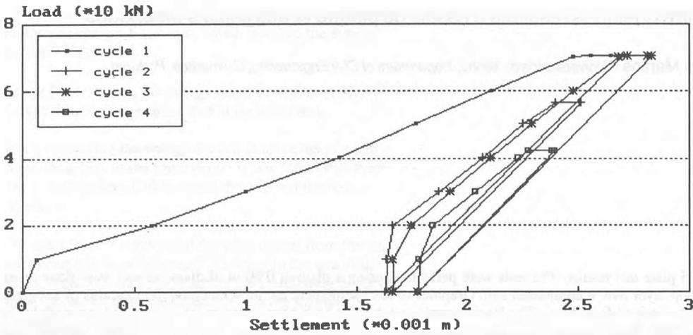
Figure 2. Load-settlement curves for the plate test PL4.
