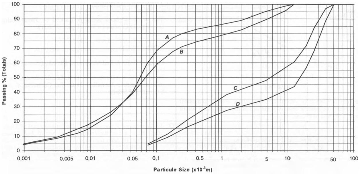
Figure 3. Grain size distribution curve for the soil foundation (A and B) and the "tout venant" (C and D).
