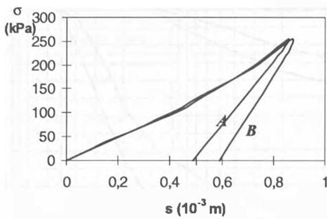
Figure 6. Curves of effective stress versus average settlement obtained in edometric tests with the soil of foundation (A - soil of site 1, B - soil of site 4).
