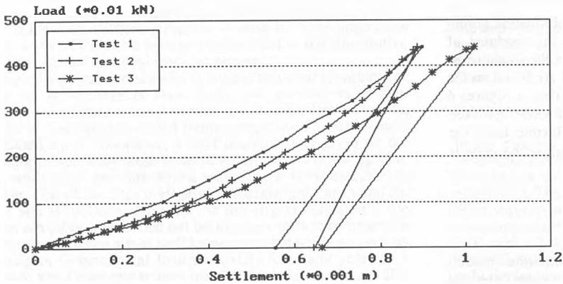
Figure 5. Load-settlement curves obtained in lab with "tout venant" of site 4.
