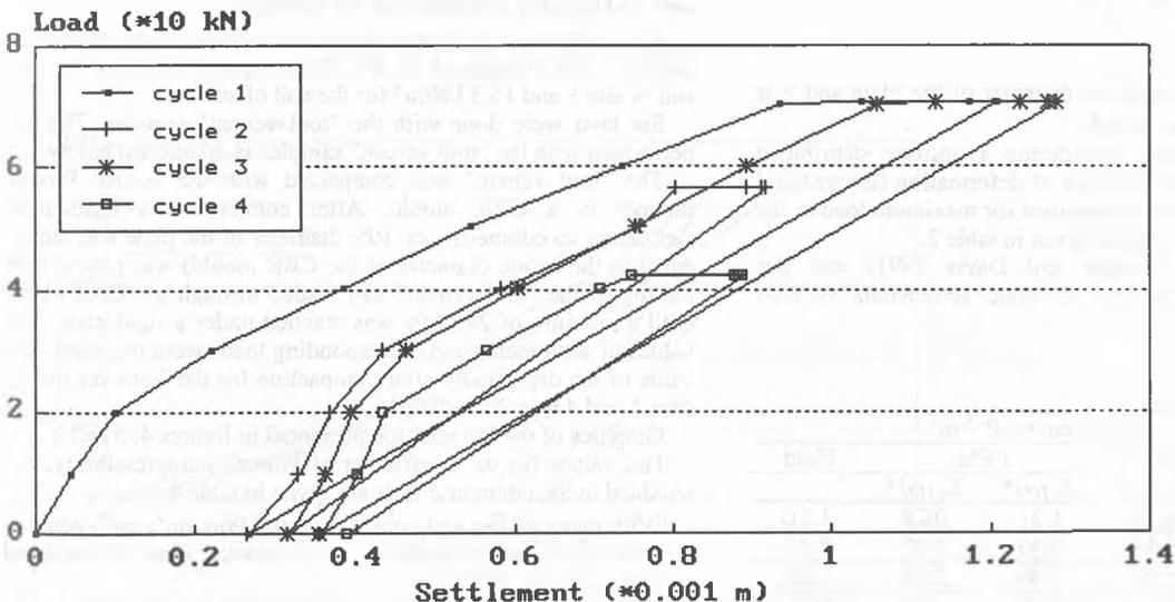
Figure 1. Load-settlement curves for the plate test PL1.
