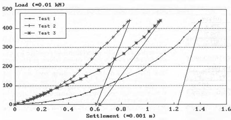
Figure 4. Load-settlement curves obtained in lab with "tout venant" of site 1.
