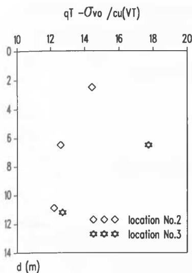
Fig.3. Cone factor for CPT shear strength
