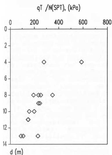
Fig.4. Corrected tip resistance related to N (SPT), all locations
