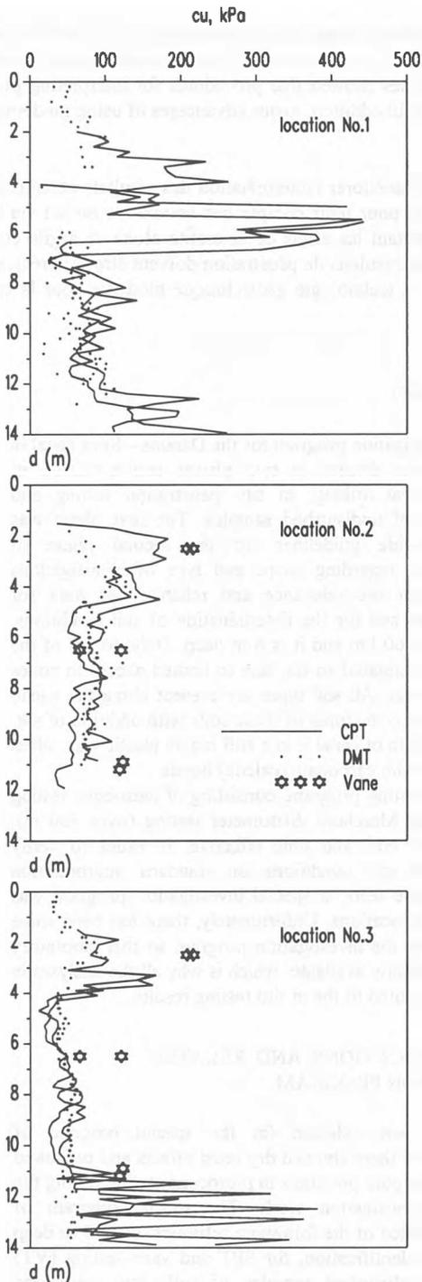
Fig. 2. Undrained shear strength profiles
