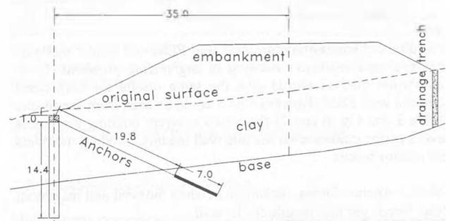
Figure 5. Typical cross-section of embankment after its renewal
