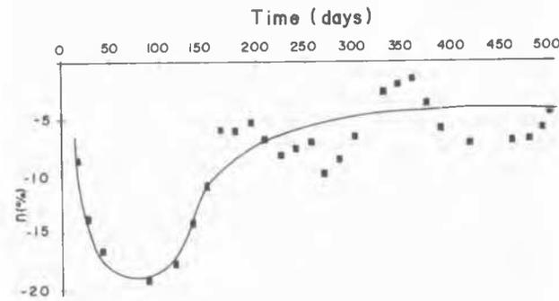
Figure 4 Load reduction by settlement readings (Inner column)
