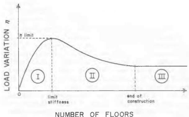
Figure 1. Variation of  $n$  during the construction
