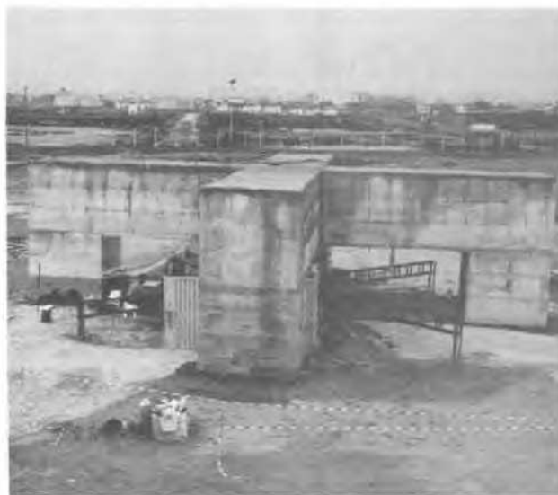
Figure 1. Pile load test arrangement
