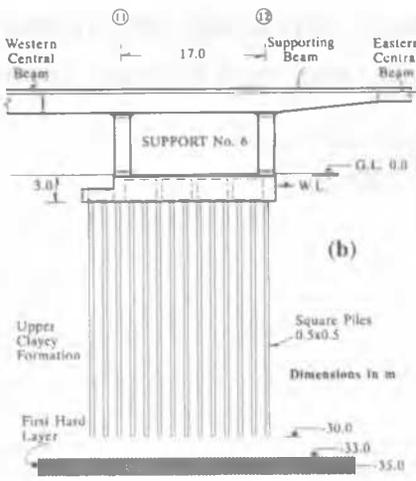
Fig 1 Geotechnical data of the site and lateral view of the instrumented mixed foundation and bridge superstructure
