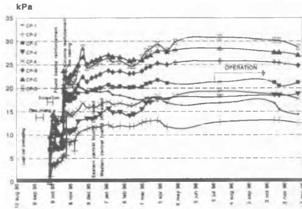
Fig 4. Measured pressures in the soil-raft contact during construction
