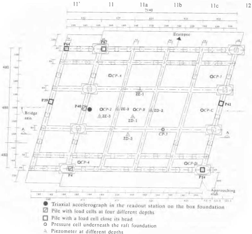
Fig 2. Plan of the instrumented friction pile-box foundation
