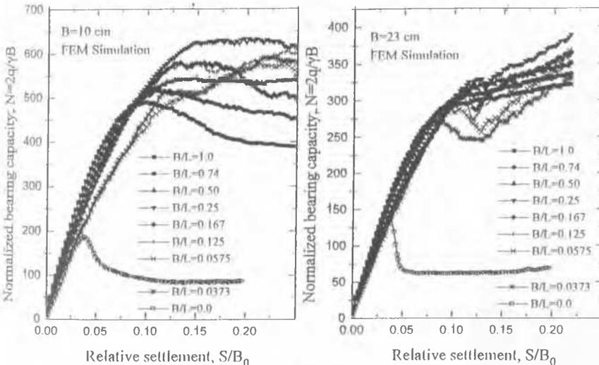
Fig. 4 Normalized load vs. relative settlement for  $B_0=10$  cm.
