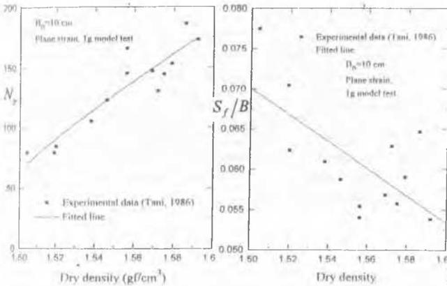
Fig. 1 Regression of  $N_\gamma$  with density. Fig. 2 Regression of  $S_f/B$  with density.
