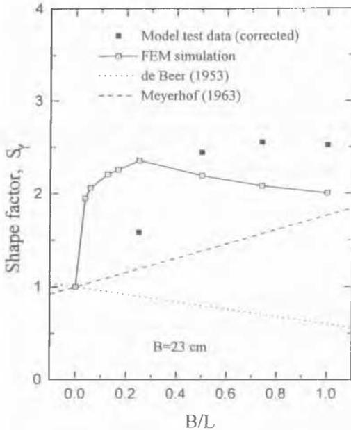
Fig. 8 Effects of shape factors ( $B_0=23$  cm)
