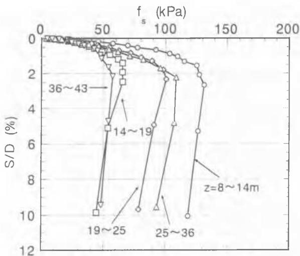
Figure 6 Relationship between the skin friction and the pile normalized settlement obtained from a full scale pile loading test
