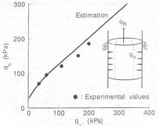
Figure 5. Comparison of bearing stresses values  $q_h$  obtained from in-situ friction tests at location T<sub>4</sub> and computed values
