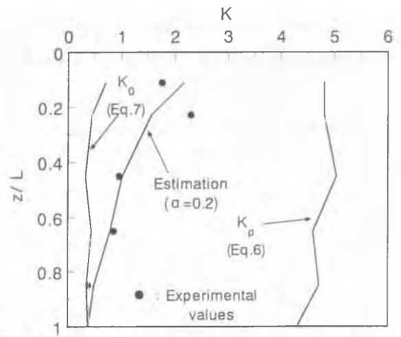
Figure 4. Comparison of lateral effective stress coefficients obtained from pressuremeter test results and computed ones
