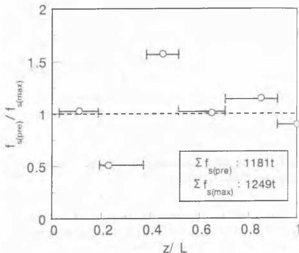
Figure 8 Ratio of the skin friction values estimated using the suggested method and measured skin friction values
