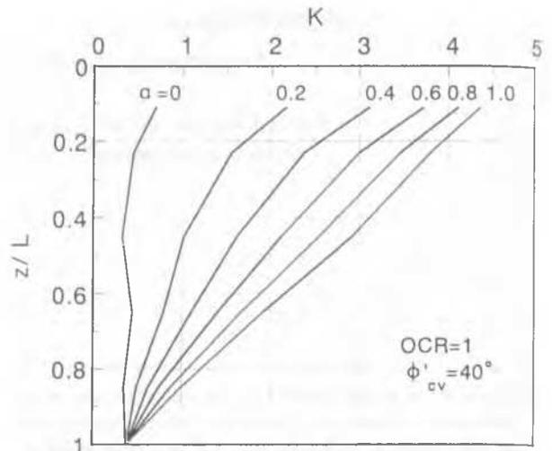
Figure 1. Variation of  $K$  with  $Z/L$  for different values of the parameter  $\alpha$
