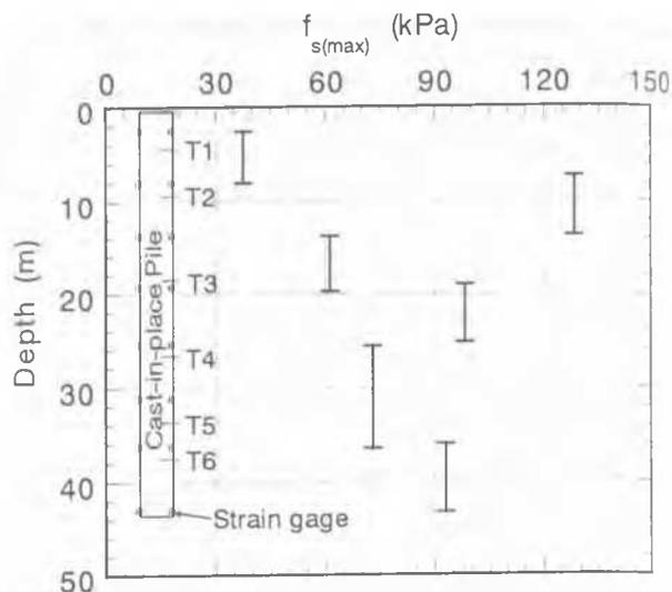
Figure 7 Relationship between maximum skin friction  $f_{s(max)}$  and the depth measured from a full scale pile loading test
