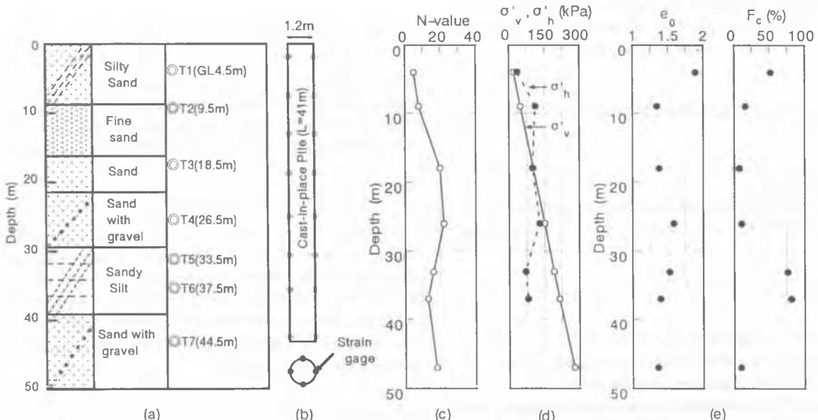
Figure 2 Soil profiles and the various soil parameters with depth for Shirasu sediments
