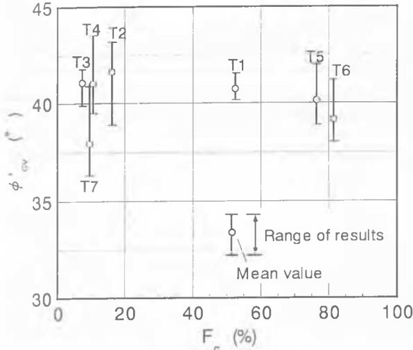
Figure 3. Relationship between  $\phi'_{cv}$  and the fines ratio  $F_c$  for the samples taken from each depth
