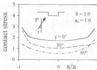
Figure 9. Contact stress distribution due to incident *P* waves.
