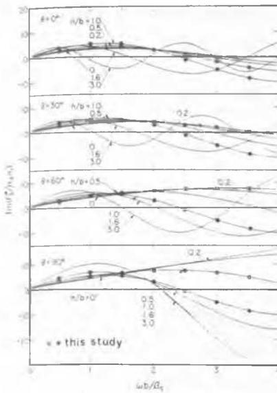
Figure 2. Imaginary part of the longitudinal driving force (Adapted from Luco et al. 1975)
