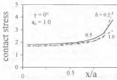
Figure 10. Effect of  $\delta$  on contact stress ( $\gamma = 0^\circ$ )
