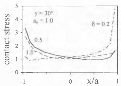
Figure 11. Effect of  $\delta$  on contact stress ( $\gamma = 30^\circ$ )
