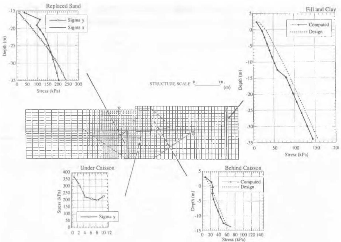
Figure 2. Computed earth pressures before the earthquake
