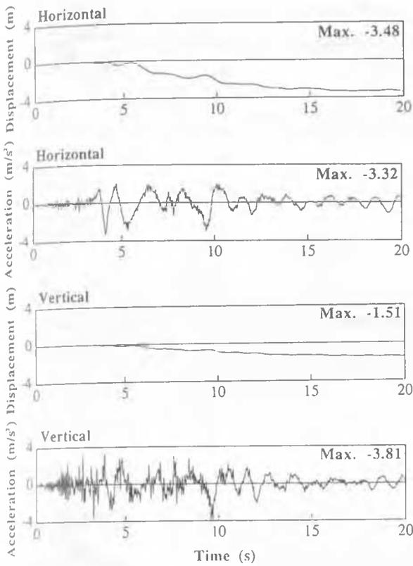
Figure 3. Computed time histories of displacements and accelerations at the sea side top corner of the caisson wall
