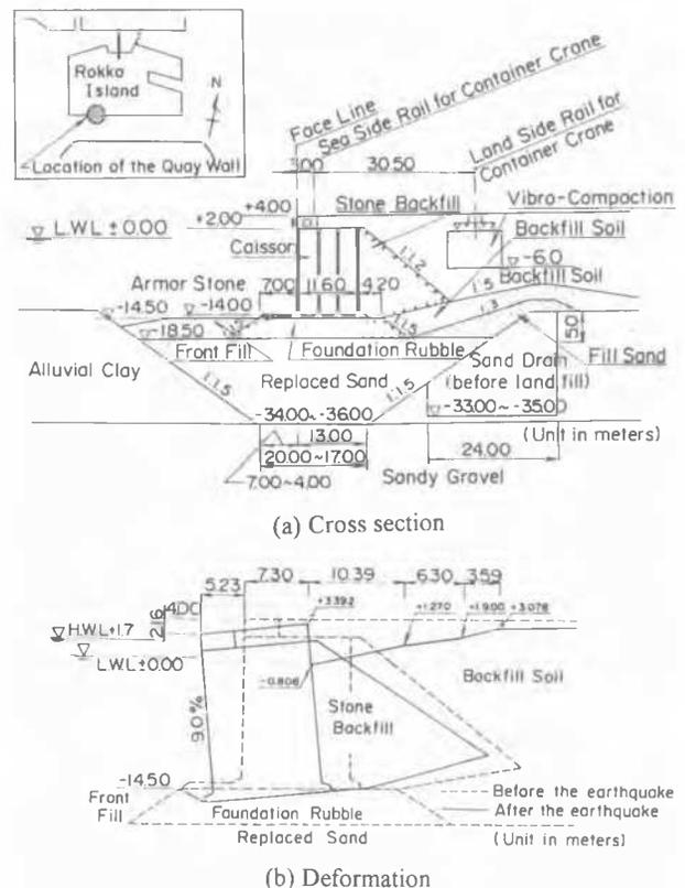
Figure 1. Cross section and deformation of a caisson wall (after Inagaki et al 1996)
