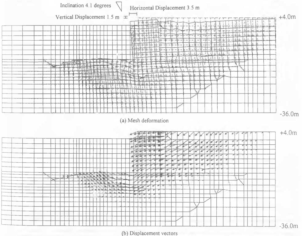
Figure 4. Computed residual displacements of caisson wall
