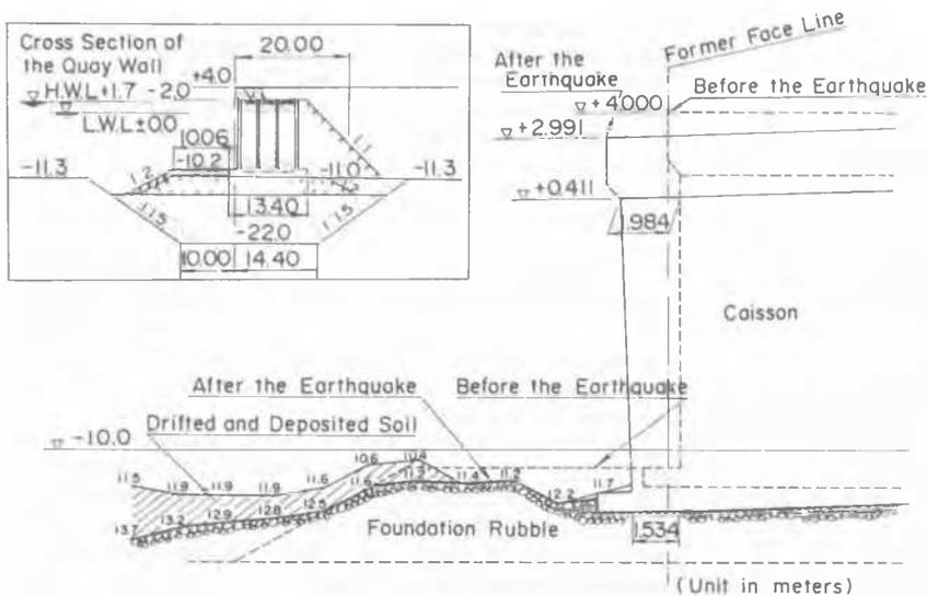
Figure 5 Deformation of rubble mound investigated by diving (after Inagaki et al. 1996)
