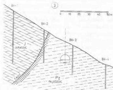
Figure 3. Characteristic cross section
