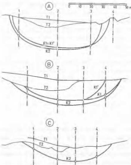
Figure 7. Cross sections A-C perpendicular to the sliding direction
