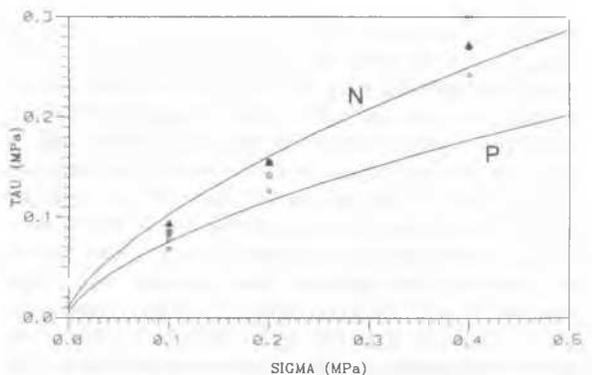
Figure 4. Drained shear strength of clastite
