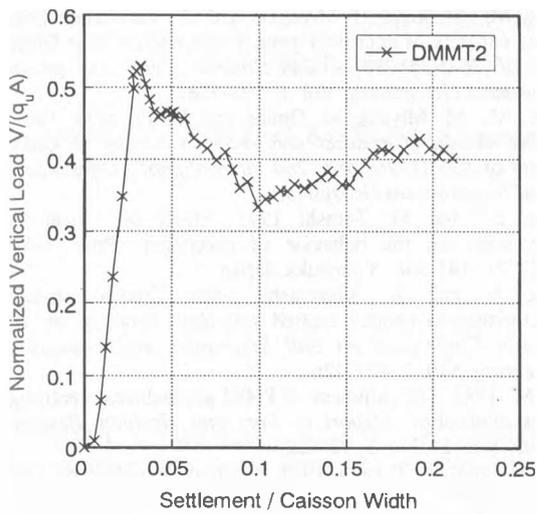
Figure 2. Load - settlement curve for vertical loading test
