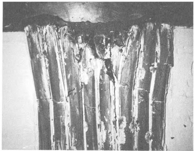
Figure 4. Failure pattern of DMM columns under vertical loading (DMMT2)
