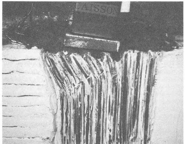
Figure 5. Failure pattern of DMM columns under inclined loading (DMMT4)
