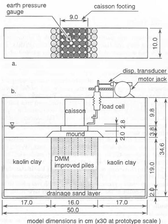
Figure 1. Model setup: a. horizontal cross-section
