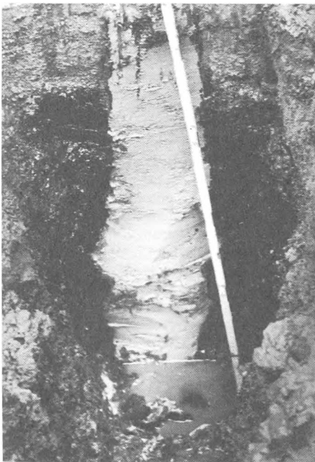
Figure 6: Result of a powder injection test in situ (peat, organic clay) using the powder lance
