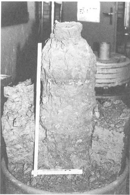
Figure 5: Result of a powder injection test on big samples (clayey silt) using the screw conveyor
