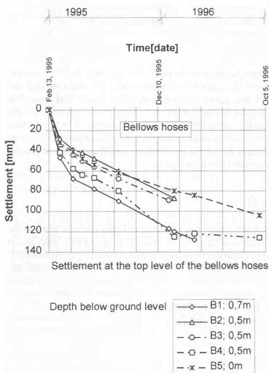
Figure 8. Follow-up of settlement with time for the upper level of bellows hoses.
