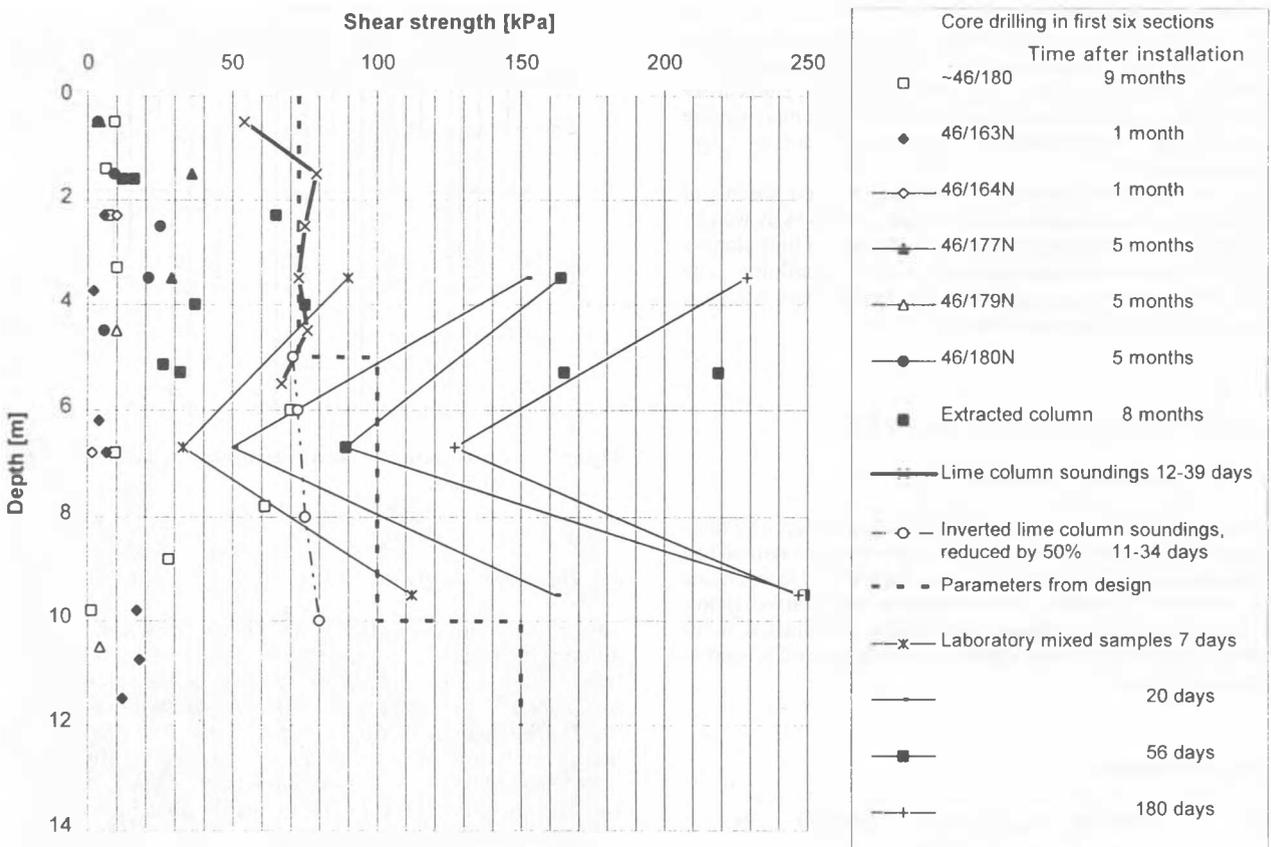
Figure 2. Diagram of shear strength against depth. Shear strength is determined by unconfined compression tests from core drilling, samples trimmed from an extracted column and laboratory mixed samples and evaluated results of soundings.
