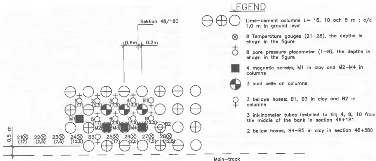
Figure 4. Measurement station at Section 46+180.
