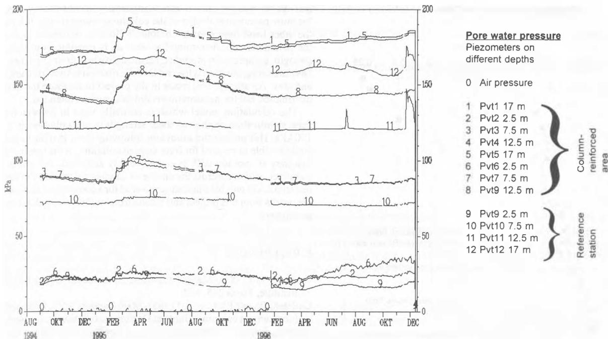
Figure 6. Pore pressure follow-up with time at different levels. Measurements carried out at a reference station and within the column-reinforced area.
