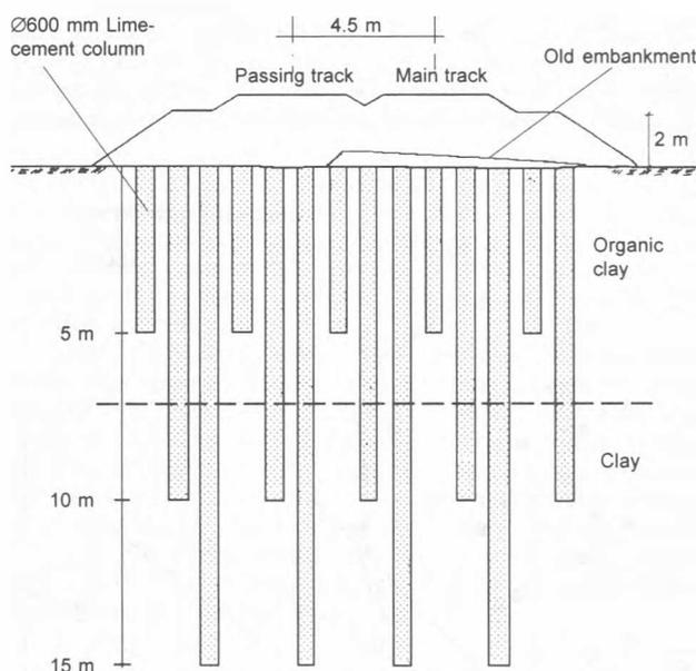
Figure 1. Cross-section of railway embankment and lime-cement columns.
