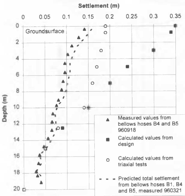
Figure 9. Measured compression in bellows hoses B4 and B5 in September 1996 and calculated compression on the basis of projected parameters or parameters chosen from triaxial tests. Prognosis of compression based on measured values in bellow hoses in March 1996.
