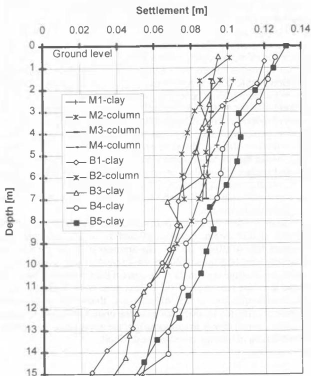
Figure 5. Measurement result for bellows hoses and magnetic screws in January 1996, 11 months after construction of the embankment.
