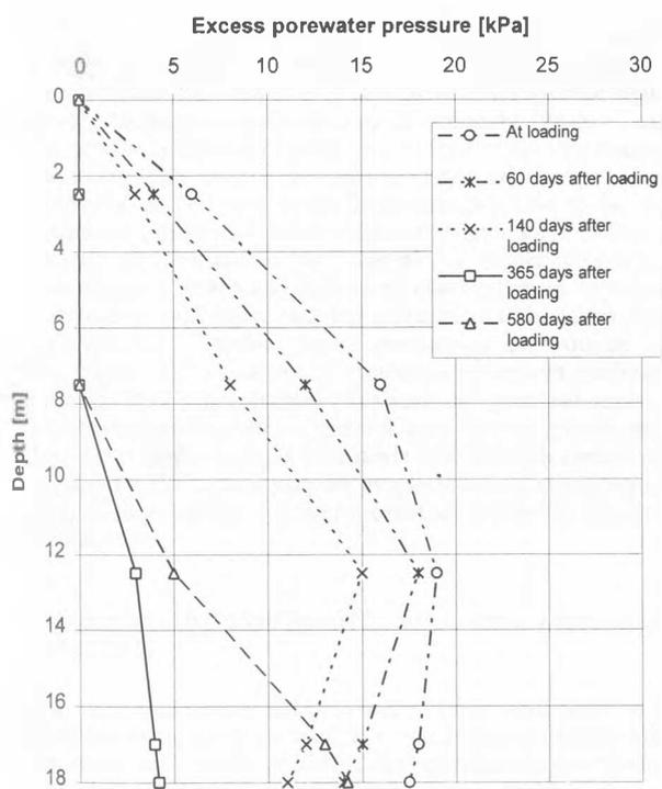
Figure 7. Distribution of excess porewater pressure in clay against depth at different points in time after loading of railway embankment.
