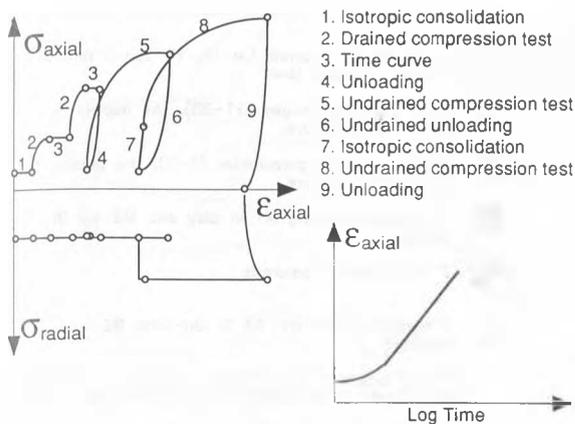
Figure 3. Schedule for carrying out triaxial tests with samples of diameter 500 mm. From Steensen-Bach et al (1996).
