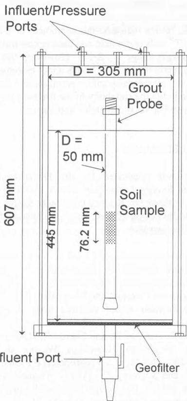
Figure 3. Diagram of the Test Column
