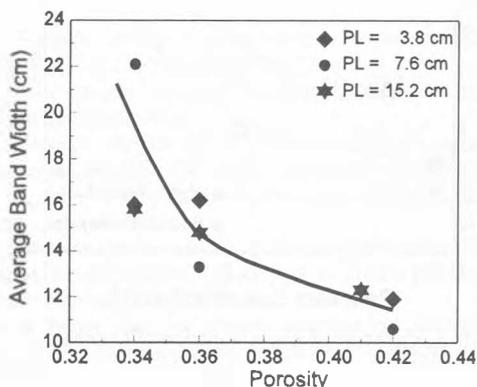
Figure 4. Variation of the Average Bulb Thickness with Soil Porosity
