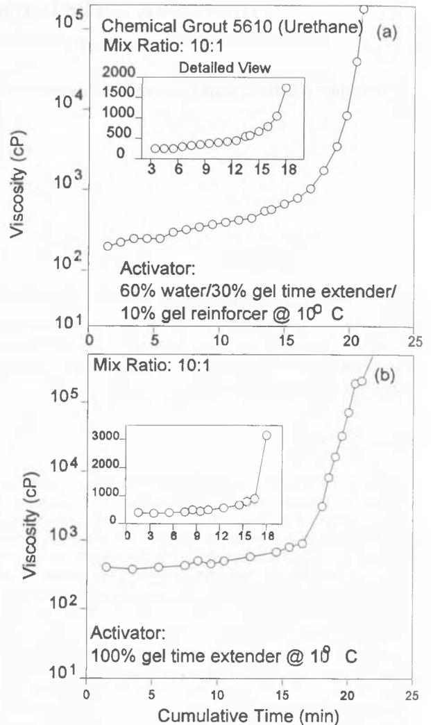
Figure 2. Variation of Viscosity with time: a) Mix 1 and b) Mix 2
