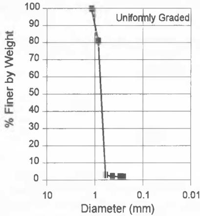
Figure 1. Grain Size Distribution of the Sand
