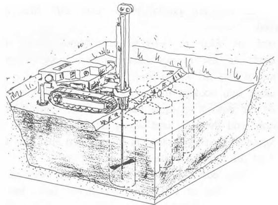
Figure 2. Typical jet-grouting pattern on a landfill
