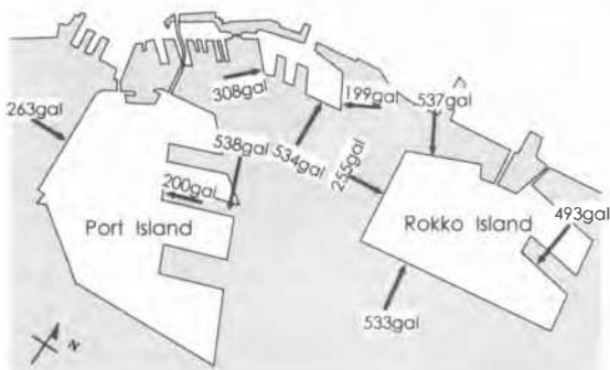
Fig. 38 Magnitude of acceleration inferred to have acted on the quaywall with different directions (Inagaki et al., 1996)
