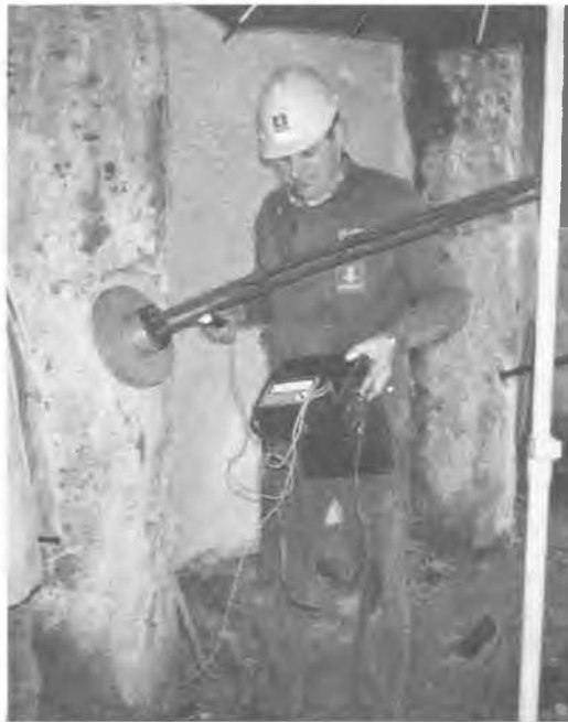
Fig. 6. Test after prestressing the anchor
