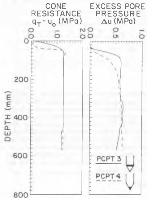
Fig. 4. PCPT profiles in specimen 2
