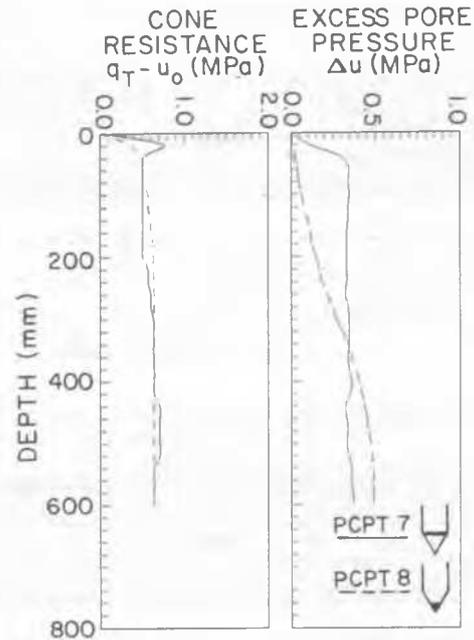
Fig. 6. PCPT profiles in specimen 4
