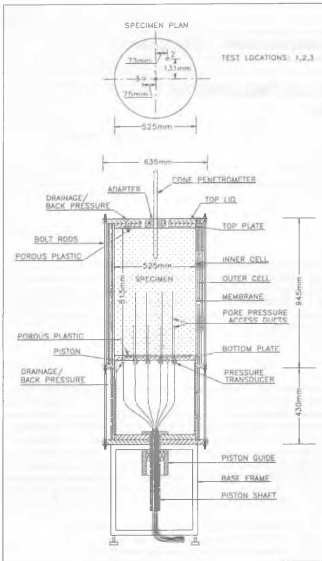
Fig. 1. Schematic of the LSU Calibration Chamber System (LSU/CALCHAS)
