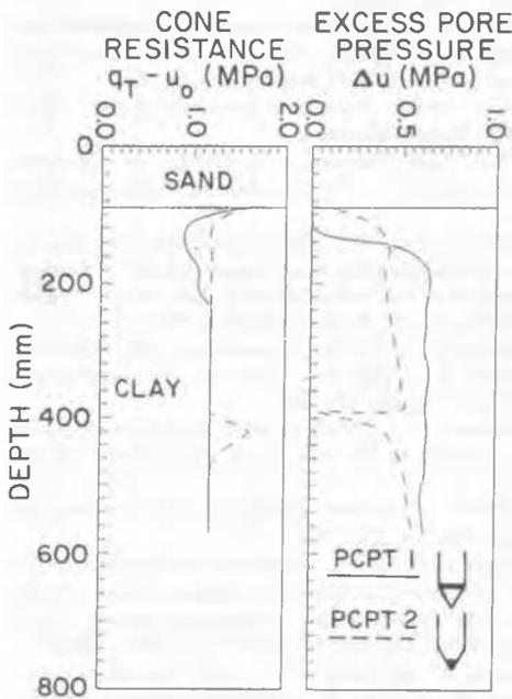
Fig. 3. PCPT profiles in specimen 1
