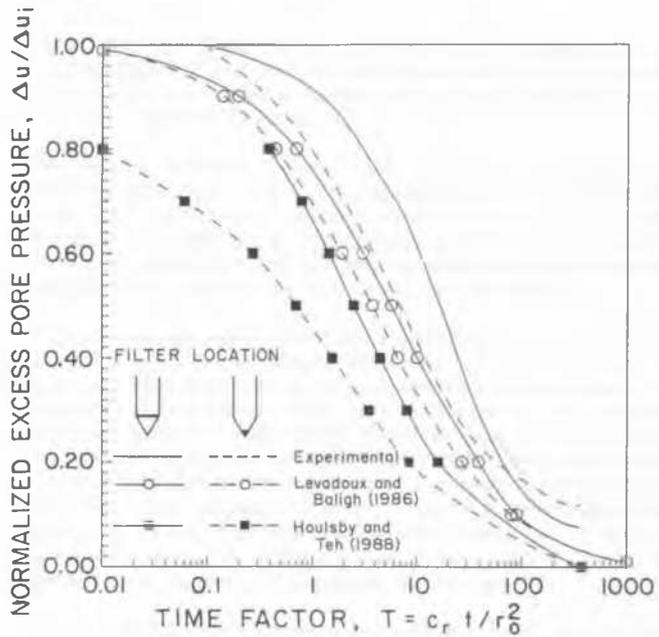
Fig. 8. Dissipation results in specimen 2
