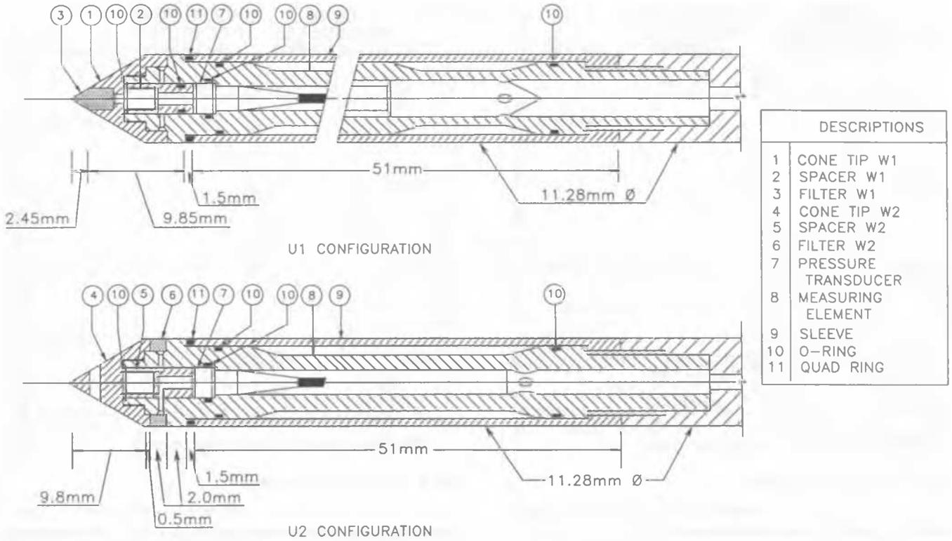
Fig. 2. Schematic of the miniature piezocone penetrometer
