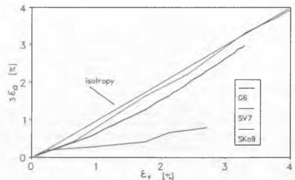
Fig 3 Examples of data from isotropic compression (loess and Gabčíkovo sand)
