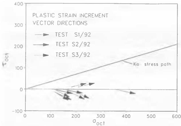
Fig 7 Results from the hydraulic cell, probes on loess specimens
