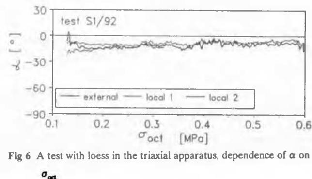
Fig 6 A test with loess in the triaxial apparatus, dependence of  $\alpha$  on  $\sigma_{oct}$
