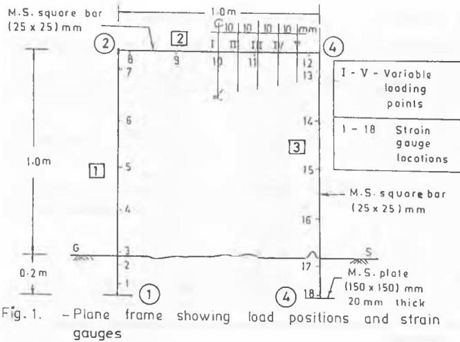
Fig. 1. - Plane frame showing load positions and strain gauges
