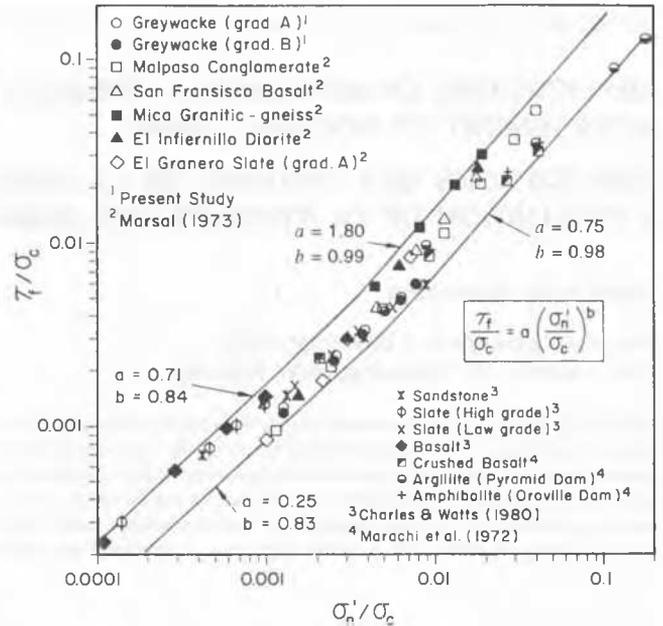
Fig. 3 Normalized Shear Strength Versus Normal Stress Response for Various Rockfill
