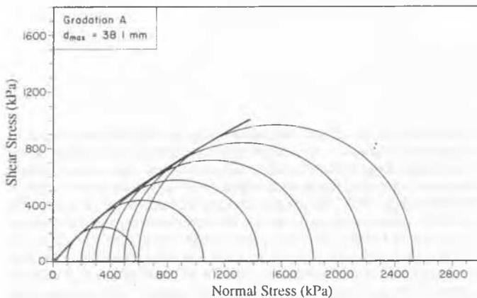
Fig. 2 Mohr-Coulomb Failure Envelopes of a Typical Greywacke Rockfill
