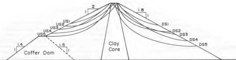
Fig. 5 Non-circular Failure Surfaces Considered in the Stability Analysis of Chiew Larn Dam
