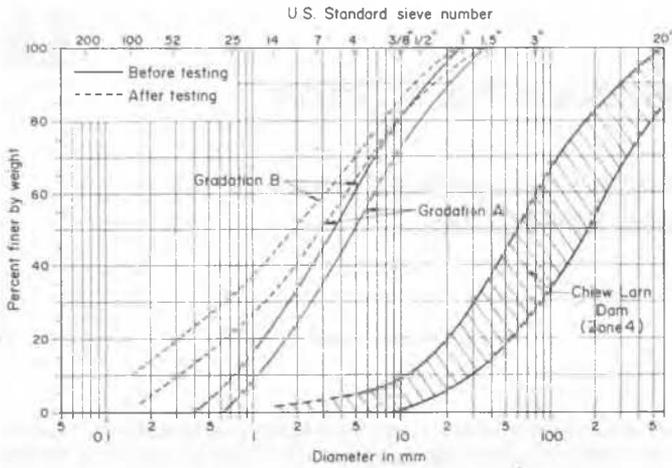
Fig. 1 Particle Size Distribution Curves of Greywacke Rockfill
