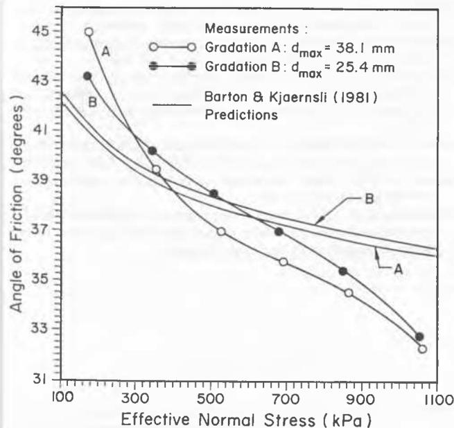
Fig. 4 Variation of Drained Angle of Friction of Greywacke Rockfill with Effective Confining Stress
