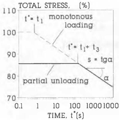
Fig. 1. The total stress-time relation given by the relaxation part-model
