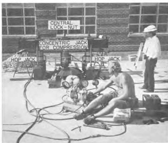
Figure 2 Tension/Compression Load Test Set-Up
