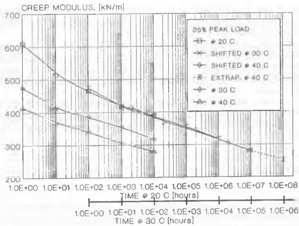
Fig. 4 Creep modulus versus time for geogrid at 20°C, 30°C and 40°C; and time-temperature superposition curve.
