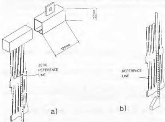
Fig. 5 a) Details for clamp for integral geogrids. b) Elongation measurement system.
