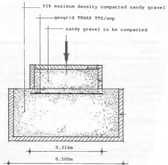
Fig. 7 Cross section of testing apparatus.
