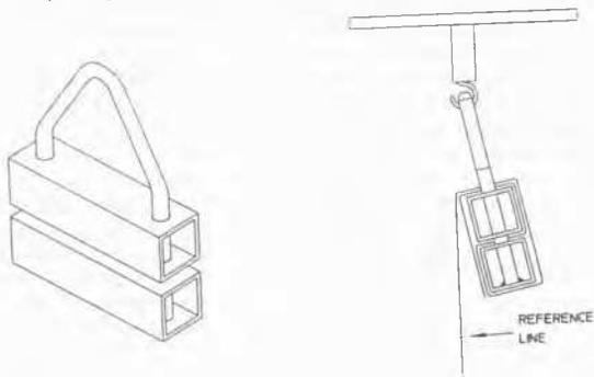
Fig. 6 Typical clamps for woven geogrid and geotextiles.
