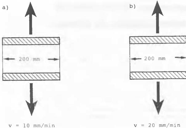
**Fig. 1.** a) ASTM D4595 wide width tensile test specimen dimensions and speed.
