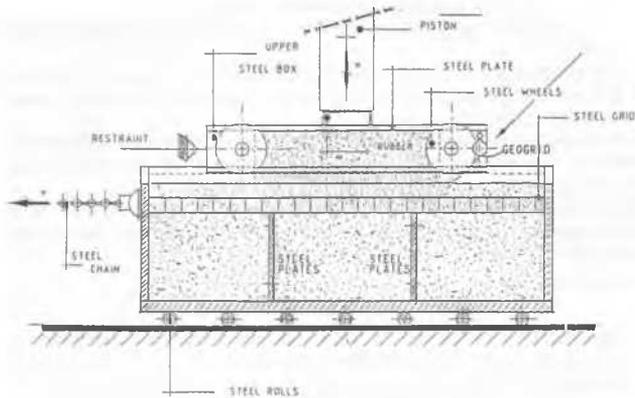
**Fig. 8** Direct shear and pullout test apparatus prepared for direct shear testing.
