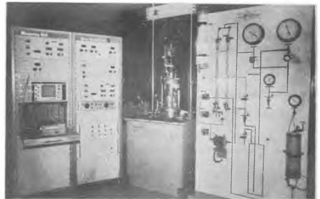
Fig.1 Overview of Cyclic Triaxial Test System
