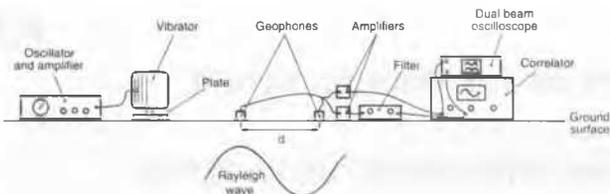
Fig 1 Rayleigh wave velocity measurement with a correlator and filter
