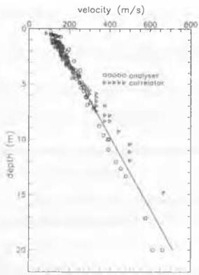
Fig 5 Comparison of correlator and spectrum analyser (Rayleigh waves)
