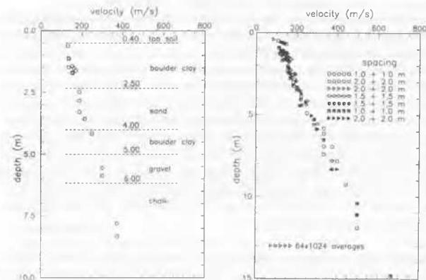
Fig 3 Soils and Rayleigh wave velocities, North Field
