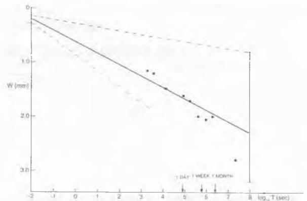
Fig 7 Calculated and observed settlement of the pad, Canons Park
