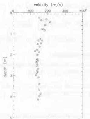
Fig 6 Rayleigh wave velocity against depth, Canons Park
