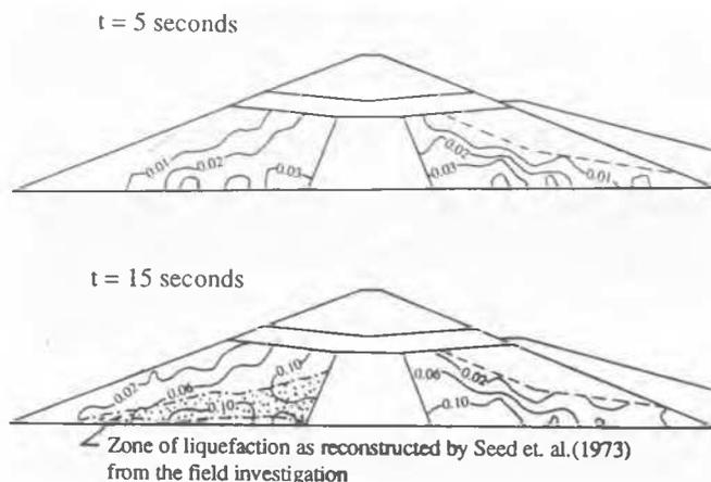
FIG. 1 Contours of probability of liquefaction in hydraulic fill after 5 sec, 10 sec, and 15 sec earthquake shaking ( $a_{max} = 0.5g$ ;  $k=0.01\text{cm/sec}$ ) -- lower San Fernando dam
