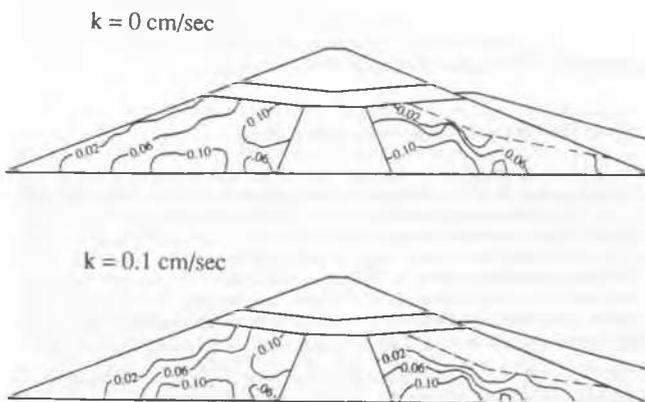
FIG. 2 Contours of probability of liquefaction in hydraulic fill for different permeability conditions ( $a_{max} = 0.5g$ ;  $t = 15$  sec) -- lower San Fernando dam
