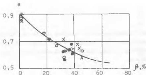
Fig. 1. Void ratio  $e$  dependence on the degree of leaching  $\beta$  for the sandy silt with  $d_0 = 26\%$  at different values of compressive stresses:
