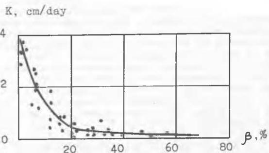
Fig. 2. Coefficient of permeability  $K$  dependence on the degree of leaching  $\beta$  at compressive stress  $\sigma_2' = 0,1$  MPa for the sandy silt with  $d_0 = 26\%$ .
