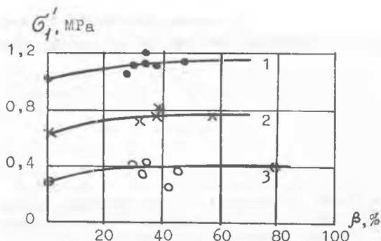
Fig. 3. Limited principal effective stresses  $\sigma_1'$  change dependence on the degree of leaching  $\beta$  and compressive stress  $\sigma_2'$  (curve 1 -  $\sigma_2' = 0,3$  MPa, curve 2 -  $\sigma_2' = 0,2$  MPa, curve 3 -  $\sigma_2' = 0,1$  MPa) at initial gypsum content  $d_0 = 26\%$ .
