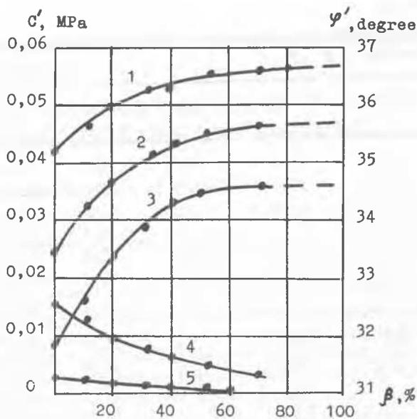
Fig. 4. Angle of internal friction  $\psi'$  (curves 1 - 3) and cohesion intercept  $C'$  (curves 4 - 5) change dependence on the degree of leaching  $\beta$  and initial gypsum content  $d_0$ . (Curves 1 and 5 -  $d_0 = 16\%$ , curve 2 -  $d_0 = 26\%$ , curves 3 and 4 -  $d_0 = 48\%$ ).
