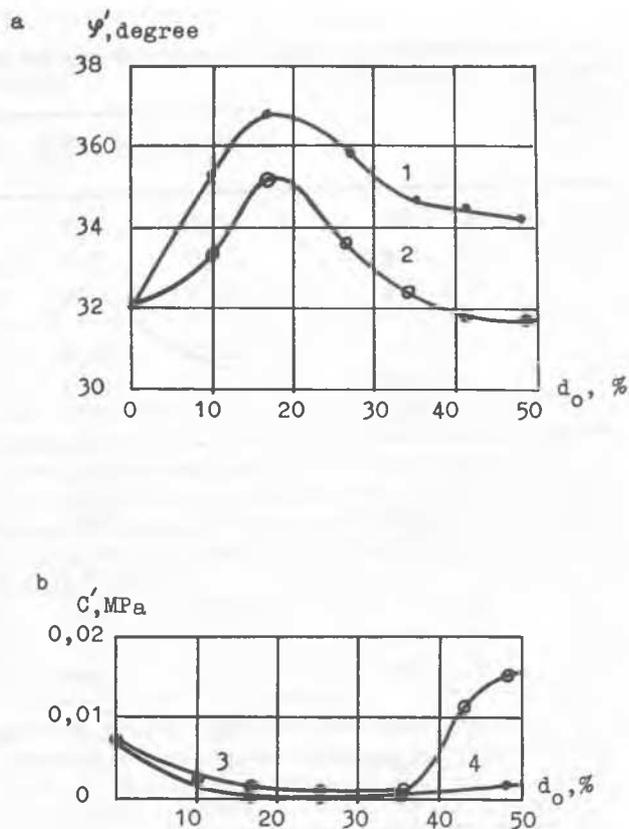
Fig. 5. Angle of internal friction  $\psi'$  (a) and cohesion intercept  $C'$  (b) dependence on the initial gypsum content  $d_0$  for the sandy silts at the nature state ( $\beta = 0$ , curves 2 and 3) and at the limiting state of desolving ( $\beta = 70\%$ , curves 1 and 4).
