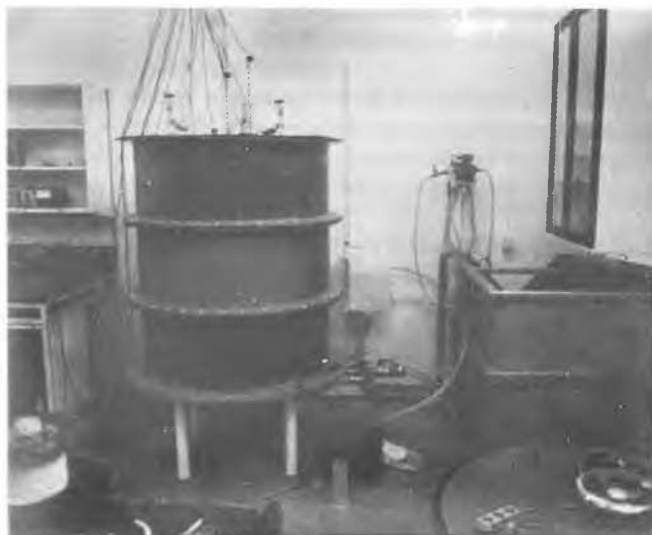
Fig. 2. Laboratory equipment used to control the accuracy and response of the field measuring instruments. Schematic (top) and during operation control test (bottom).
