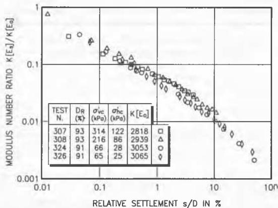
**Fig. 3.** Modulus number of very dense NC dry Ticino Sand from deep plate loading tests performed in Calibration Chamber.
