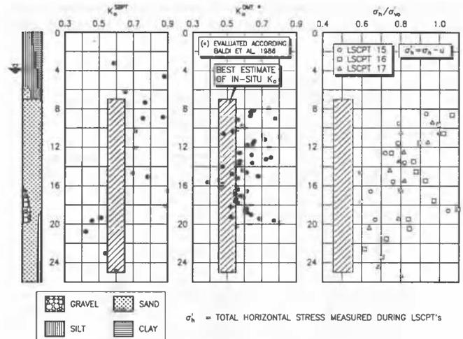
**Fig. 5.** Coefficient of earth pressure at resp of Po River sand from SBP and DM tests.
