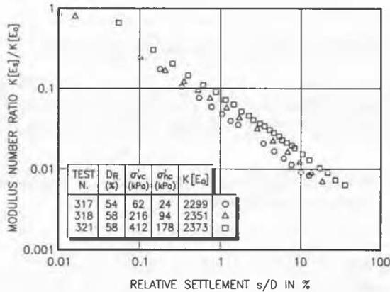
**Fig. 2.** Modulus number of medium dense NC dry Ticino Sand from deep plate loading tests performed in Calibration Chamber.
