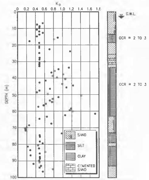
Fig. 7. Coefficient of earth pressure at rest from seismic tests.
