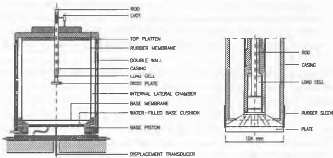
Fig. 1. Plate loading tests in Calibration Chamber.
