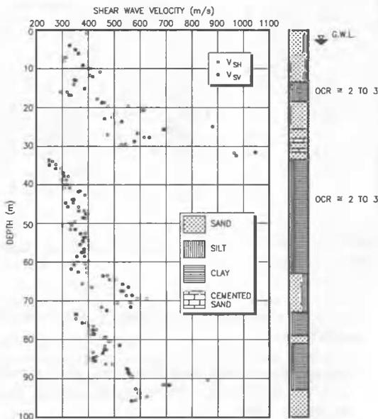
Fig. 6. Horizontally and vertically polarized shear waves
