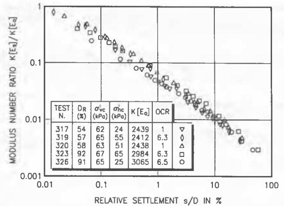
**Fig. 4.** Modulus number of medium dense NC and OC Ticino Sand from deep plate loading tests performed in Calibration Chamber.
