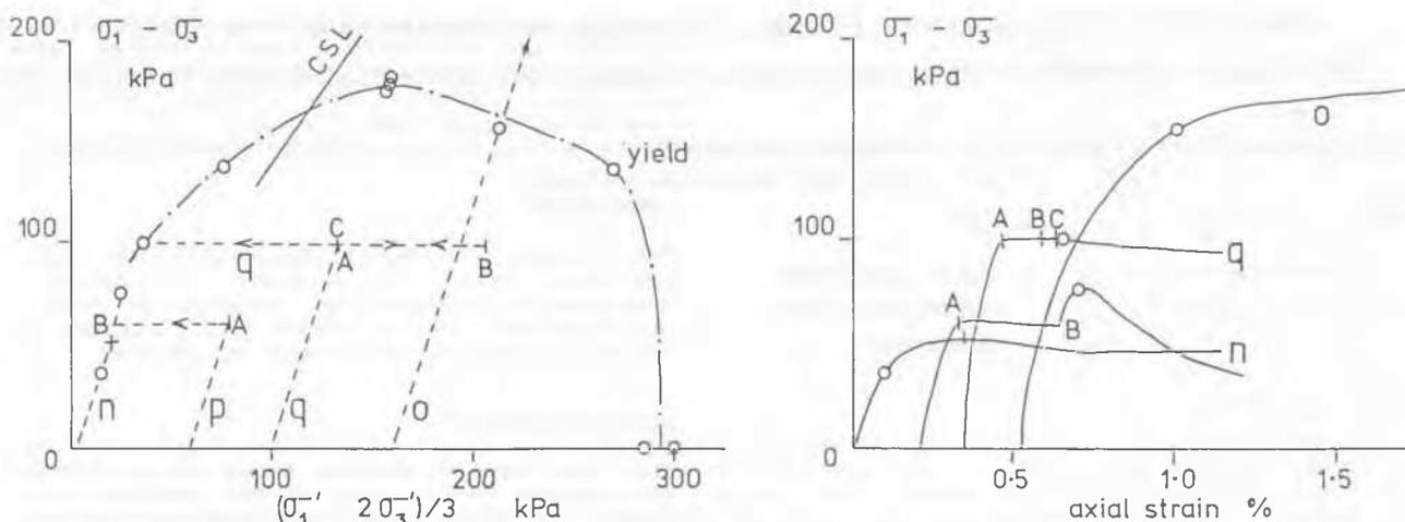
Figure 3. The effect of stress path on yield and failure of artificial bonded soil; 57%  $q_s$ , 30%  $k_s$ , 13%  $k_b$ , fired for 5 hours at 500°C.
