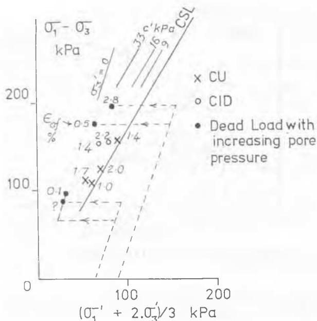
Figure 4. Failure of residual soil from granite in drained [CID], consolidated undrained [CIU], and dead load triaxial tests [Geotechnical Control Office, 1982].
