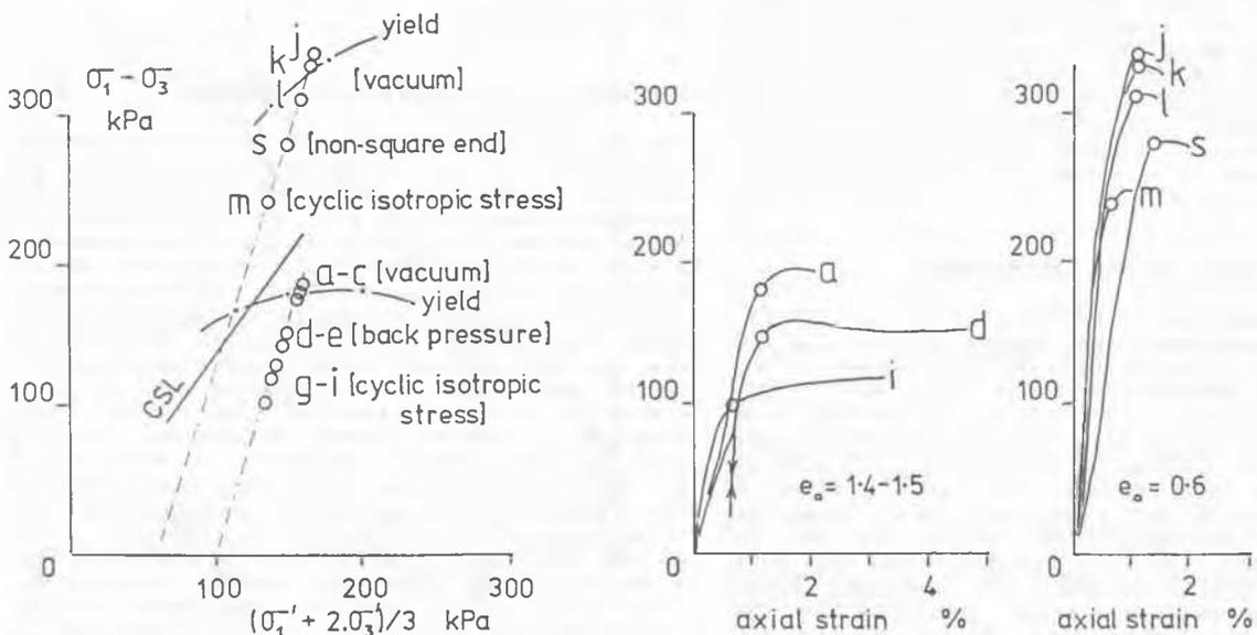
Figure 2. The effect of saturation method and non-square ends on yield and failure of artificial bonded soil. Tests a - i : 57% qs, 30% ks, 13% kb; tests j - m: 87% qs, 13% kb; all fired for 5 hours at 500 °C.
