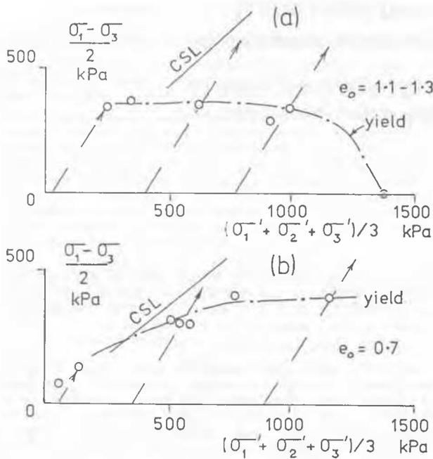
Figure 1. Yield of [a] residual soil from Basalt, [b] artificial soil [57% qs, 30 % ks, 13% kb, fired 500°C for 5 hours]. [After Vaughan *et al*, 1988].
