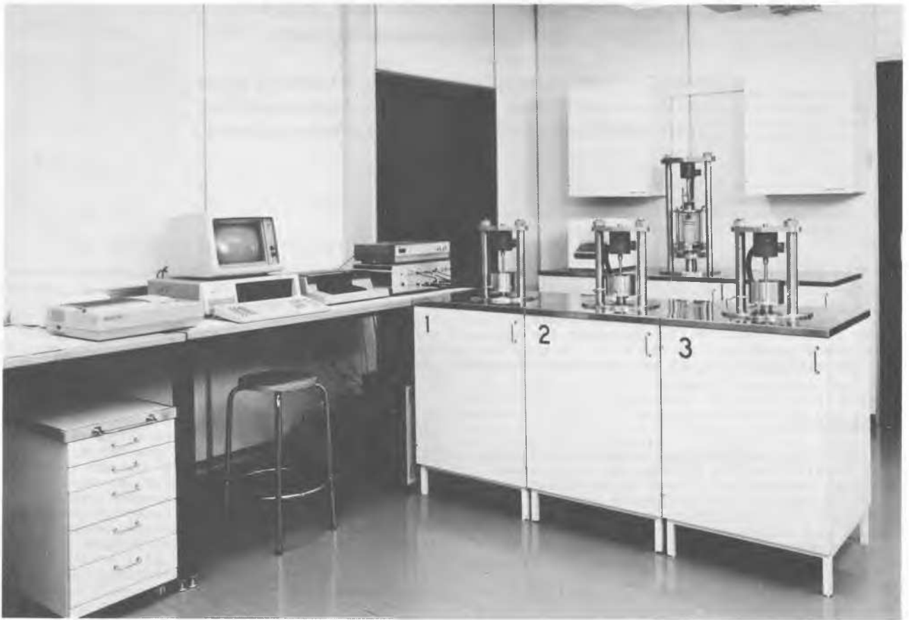
Figure 1. The new triaxial-oedometer device; the three oedometer units in the foreground and the triaxial unit at the back.
